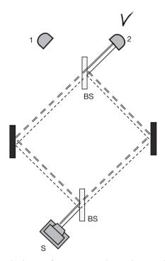
Figure 4. A Mach–Zehnder interferometer, tuned in such a way that all particles from S go to the port 2.
