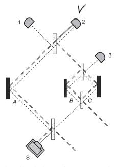
Figure 5. The internal Mach–Zehnder interferometer is tuned in such a way that the particle cannot go from source S to detector 2 through the right arm. Nevertheless, at B both forwards and backwards evolving states are present, and for any weak coupling to the particle at B, the effect is as if there were a single particle there.
