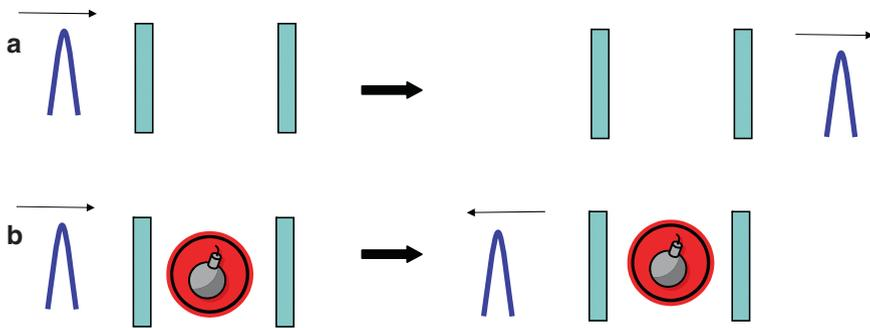
**Fig. 3** The Paul and Pavičić scheme. (a) If the cavity is empty, the photon passes through it with very high probability. (b) If the object is present in the cavity, the photon is reflected with very high probability
