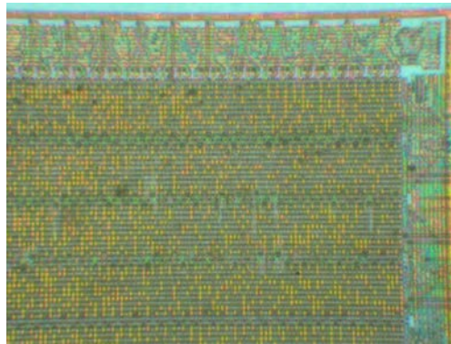
NEC \mu PD78F9116 microcontroller 0.35 \mu m
