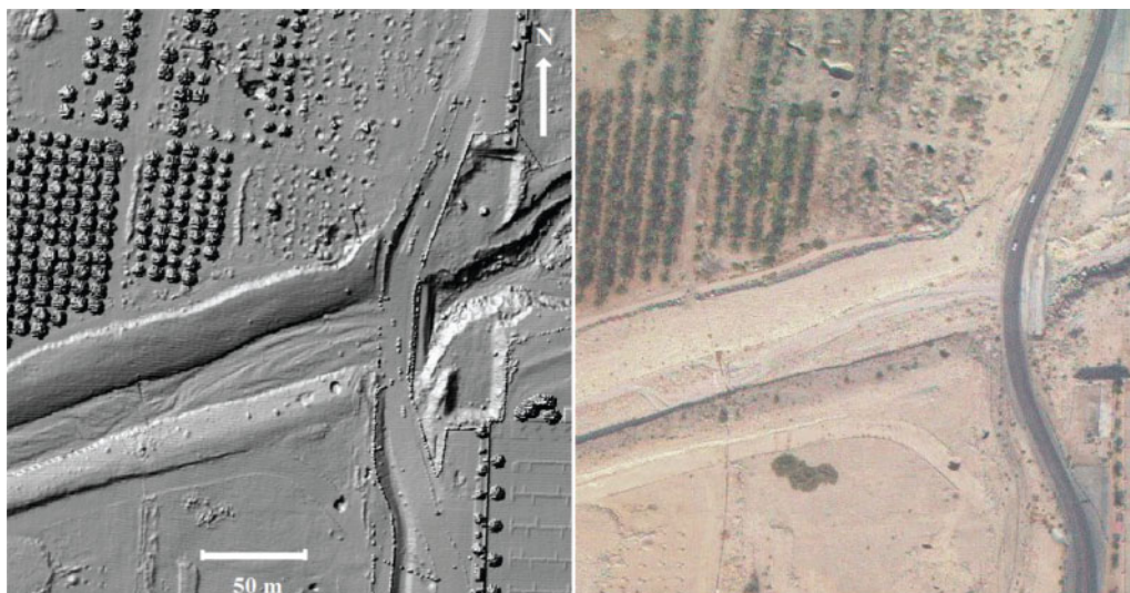
5 Comparison of image and laser data: notice the clear expression of the sinkholes in the laser data contrasting the difficulty in distinguishing them in the aerial image as well as separating them from shrubs and rocks
