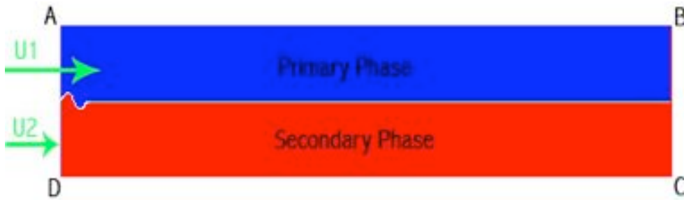
Figure 25 Illustration of the phases and boundary conditions in CFD model. Sheared velocity inlet on edge AD ( U1 and U2 ), along with a sinusoidal perturbation. Upper layer set to be the primary phase (the lighter layer) and the heavier layer set to be the secondary phase. Edge BC is set to pressure outlet boundary.
