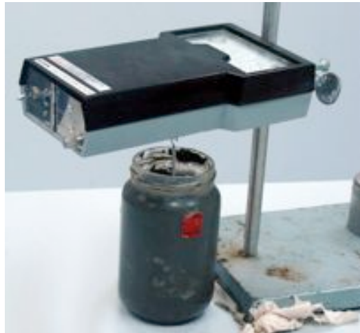
Figure 24 Viscosity measurements by viscometer. The jar is filled with Ze'elim formation's mud from "Mineral Beach", Dead Sea. A rotor is inserted into the sample, rotating at 62.5 rpm. Measured viscosity \sim 0.3 - 3 Pas.
