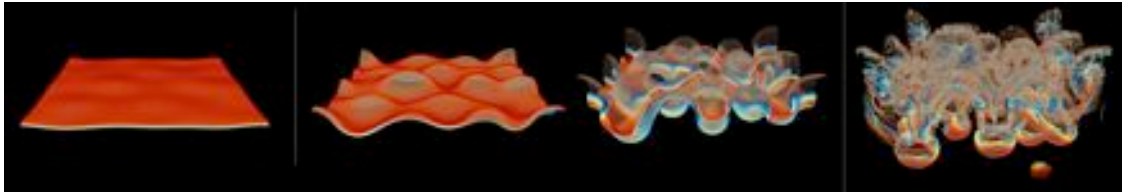
Figure 32 Numerical simulation of Rayleigh-Taylor instability. This sequence shows four time intervals from an XT3 simulation (on a 768^2 \times 1536 grid), with regions of predominantly heavier fluid (red), lighter fluid (blue). By the time of the fourth image the mixing shows descending “mushroom caps” that produce fine-scale mixing. Note the visual likeness of the mushroom-cups to the folded sediments of the Lisan Formation. By a vertical incision the density interface may look similar to the exposed billow-like folds of the Lisan Formation.
