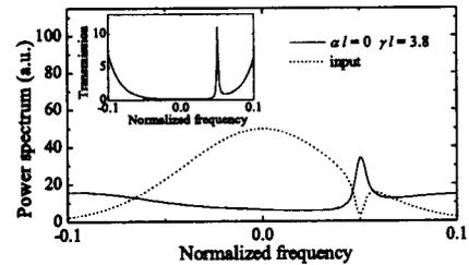
Fig. 12. Calculated spectra for the experimental parameters of Fig. 5. Inset, normalized transmission.
