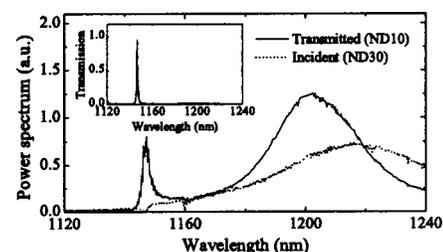
Fig. 4. Incident and transmitted spectra for GaAs at high power ( $2\text{-}\mu\text{J}$  pulse energy), with the laser tuned to 1220 nm (300-g/mm grating). Inset, normalized transmission.  $\text{ND}_x$  refers to the neutral-density filter used in each measurement.
