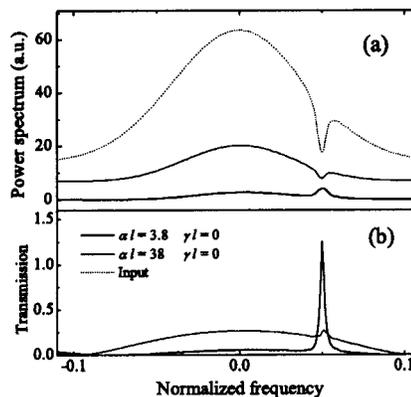
Fig. 9. Calculated spectra for a medium characterized by a purely dissipative nonlinearity ( $\gamma = 0$ ). (a) Transmitted power spectra, (b) the corresponding normalized transmission curves. The dashed curve in (a) is the power spectrum at the input of the nonlinear medium. The curves in (a) are displaced vertically in steps of 7 a.u. to improve clarity.
