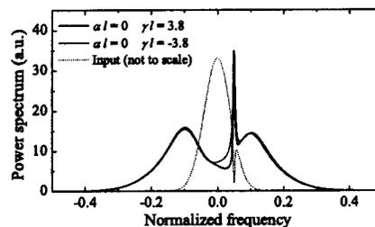
Fig. 8. Calculated transmitted power spectra for a pure Kerr medium ( $\alpha = 0$ ). The dashed curve is the power spectrum at the input of the nonlinear medium.
