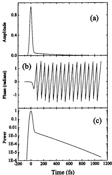
Fig. 7. Modified temporal shape of an input Gaussian pulse after it propagates through a linear absorber characterized by the transfer function shown in Fig. 6. (a) Amplitude of the modified pulse, (b) the pulse's time dependent phase. The absolute square of the complex envelope function is depicted in (c) on a logarithmic scale. Note the weak exponential tail trailing behind the pulse.
