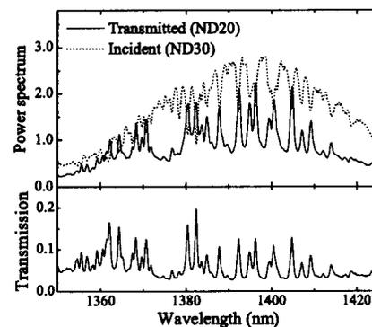
Fig. 3. Spectra for GaAs at high power ( $2\text{-}\mu\text{J}$  pulse energy) with the laser tuned to 1400 nm (300-g/mm grating). Top, incident and transmitted spectra; bottom, normalized transmission.  $\text{ND}_x$  refers to the neutral-density filter used in each measurement.
