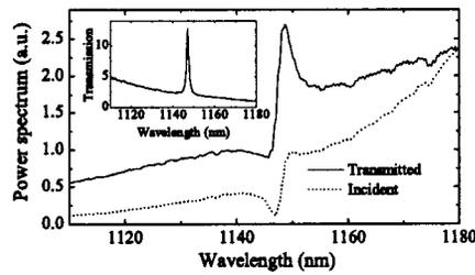
Fig. 5. Incident and transmitted spectra for glass at high power ( $2\text{-}\mu\text{J}$  pulse energy) with the laser tuned to 1220 nm (300-g/mm grating). Inset, normalized transmission.
