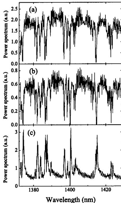
Fig. 2. Incident and transmitted spectra for InP, with the laser tuned to 1400 nm (1200-g/mm grating): (a) incident spectrum, (b) transmitted spectrum at low input intensity ( $0.02\text{-}\mu\text{J}$  pulse energy), (c) transmitted spectrum at high input intensity ( $2\text{-}\mu\text{J}$  pulse energy).
