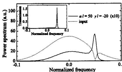
Fig. 11. Calculated spectra for the experimental parameters of Fig. 4. Inset, the normalized transmission.
