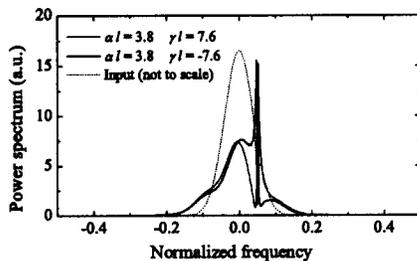
Fig. 10. Calculated transmitted power spectra for a medium with both nonlinear absorption and a nonlinear refractive index. The dashed curve is the power spectrum at the input of the nonlinear medium.
