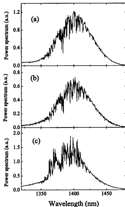
Fig. 1. Incident and transmitted spectra for InP, with the laser tuned to 1400 nm (300-g/mm grating): (a) incident spectrum, (b) transmitted spectrum at low input intensity ( $0.02\text{-}\mu\text{J}$  pulse energy); (c) transmitted spectrum at high input intensity ( $2\text{-}\mu\text{J}$  pulse energy).
