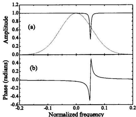
Fig. 6. Complex spectral transfer function of a Lorentzian absorption line. (a) Amplitude of the transfer function superimposed upon the input spectrum, (b) phase of the transfer function (the parameters are given in the text).
