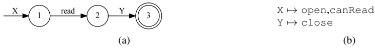
Fig. 4 (a) Symbolic automaton representing the query for the behavior around the method read and (b) the assignment to its symbolic transitions which answers the query.
