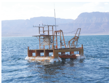
FIGURE 2: The Dead Sea hydrometeorological buoy.
