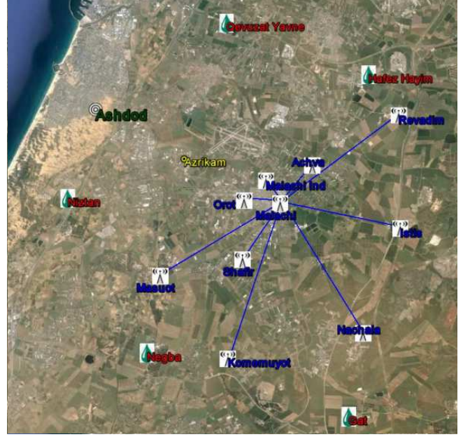
Fig. 1. The test area. The MWL system (blue lines) is shown beside the RH gauges (green drops) and the LWS (at Azrikam).
