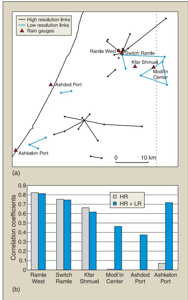
**Fig. 5.** Integration of data from multiple networks: (a) A map of the area with HR links marked in black, LR links in blue, and rain gauges are noted by red triangles (MATLAB). (b) The correlation coefficients between rain gauge and microwave link measurements.
