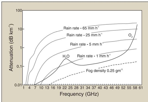
Fig. 2. A graph of transmission losses in the atmosphere.
