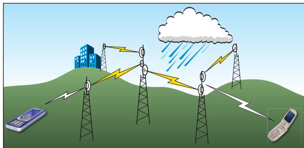
**Fig. 1.** A microwave network using fixed wireless electromagnetic communication links between the base stations that operate at frequencies of tens of GHz. Rainfall is the major source of communication impairments.
