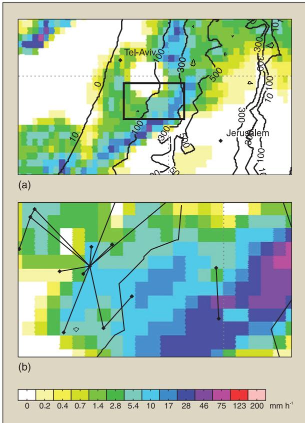
**Fig. 4.** (a) A rainfall intensity field produced by weather radar. (b) Rainfall measured directly near the ground by constructing data from microwave multiple links over the selected area in (a) (MATLAB).
