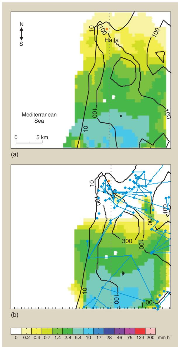
**Fig. 3.** (a) A rainfall intensity field produced by weather radar. (b) The same rainfall field reconstructed from simulated multiple microwave links data (MATLAB). The black contours are geographic elevations in meters above sea level.
