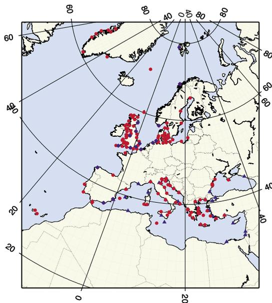
Fig.2 The European Sea Level Service Network. Red dots are tide gauges. Blue diamonds are tide gauges with co-located CGPS. Blue triangles are designated MedGLOSS sites which are available to ESEAS through coordination with MedGLOSS. The North African coasts do not have a sufficient network. Plans to update them are in progress (Fig.1).
