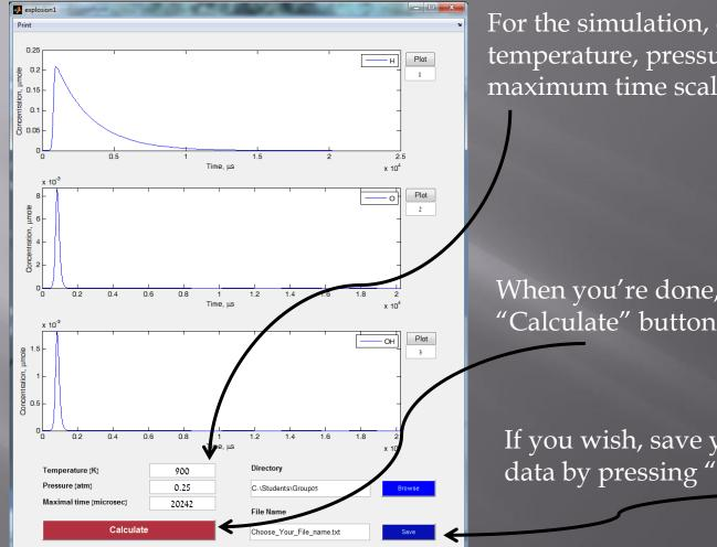
For the simulation, enter temperature, pressure and maximum time scale
