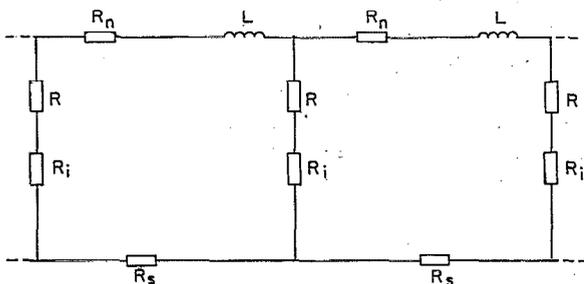
FIG. 2. Effective electrical circuit describing the current distribution in the composite superconductor.
