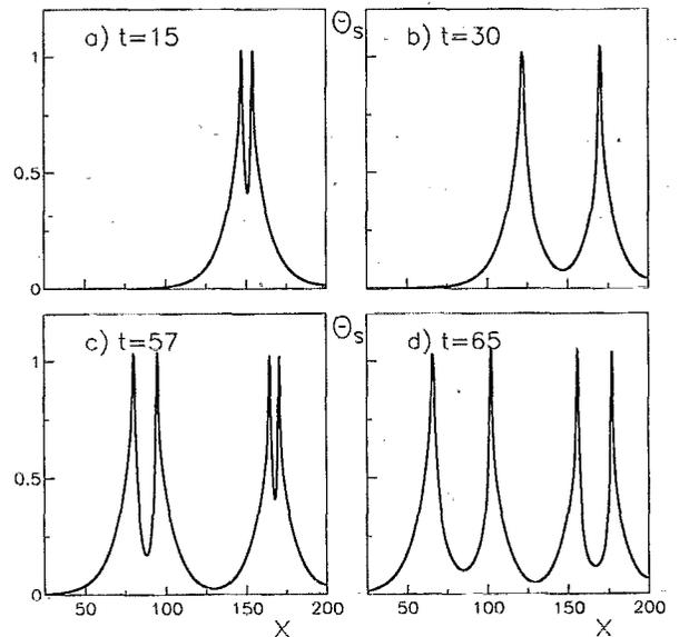
FIG. 6. The dynamics of temperature distribution in the superconductor,  $\theta_s$ , in the case of a string of resistive domains. The parameters are  $\lambda=20$ ,  $\tau_m=2$ ,  $i=0.6$ .
