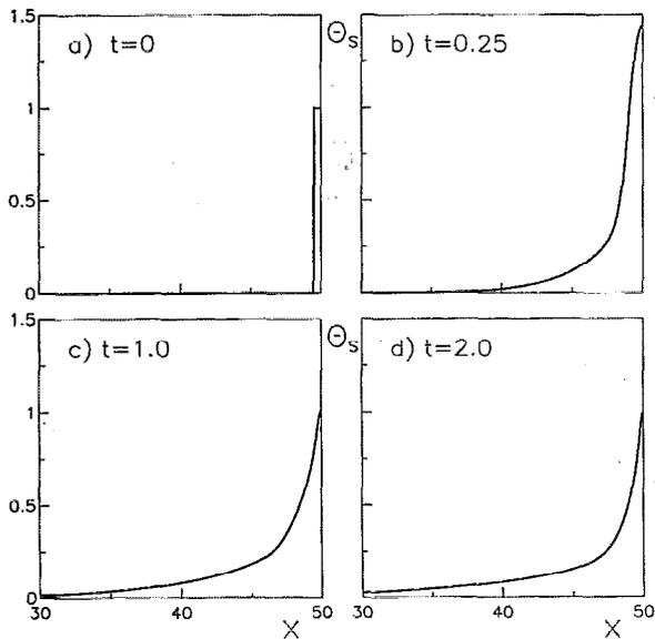
FIG. 4. The dynamics of temperature distribution in the superconductor,  $\theta_s$ , in the case of a resistive domain. The parameters are  $\lambda=20$ ,  $\tau_m=3$ ,  $i=0.3$ .
