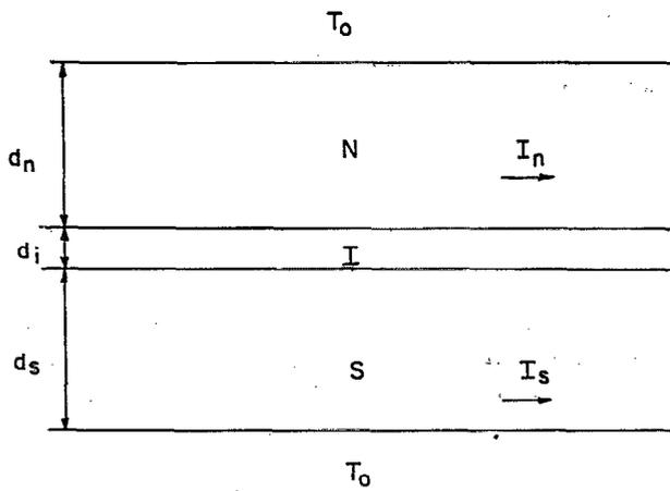
FIG. 1. Schematic structure of the considered composite superconductor.
