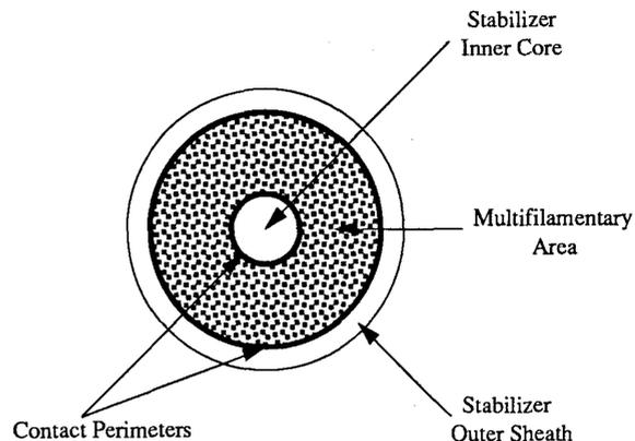
Figure 1: The conductor cross-section.
