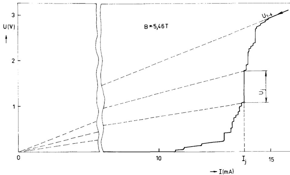
Figure 8 Recovery part of current-voltage characteristics measured between taps 1 and 6 in magnetic field  $B = 5.46\text{ T}$
