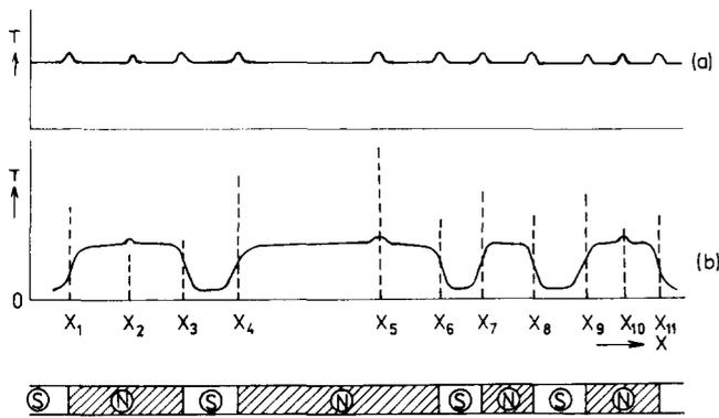
**Figure 4** Temperature distribution along the superconductor with point inhomogeneities during the recovery of superconductivity: (a)  $T(x)$  at  $I > I_p$ ; (b) possible temperature profile  $T(x)$  at  $I < I_p$  and corresponding distribution of normal and superconducting zones along a filament. - - -, Positions of hot points. The length of each dashed line is proportional to the corresponding value of  $\Gamma$
