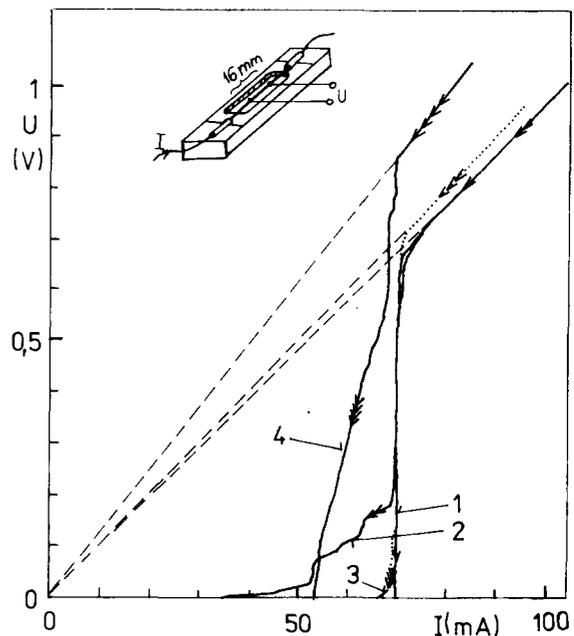
**Figure 5** Recovery part of voltage-current characteristics of the bare  $36 \mu\text{m}$  Nb-Ti filament: 1, original sample; 2, sample covered with thin layer of GE varnish over a length of  $\approx 5$  mm between the potential taps; 3, sample without GE varnish, slightly etched over a length of  $\approx 2$  mm; 4, sample without GE varnish, etched a little more over a length of  $\approx 10$  mm. Insert, sample and sample holder
