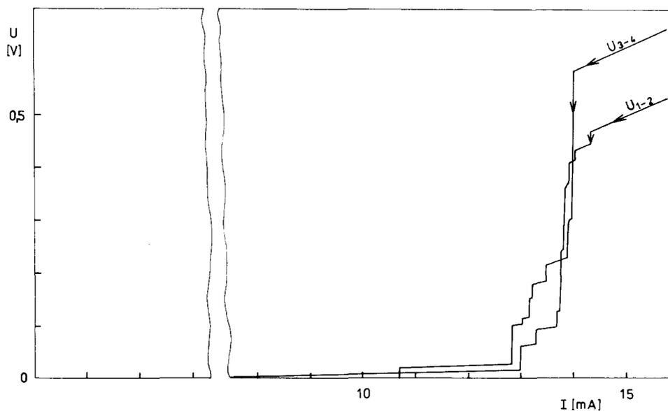
Figure 9 Recovery parts of current-voltage characteristics measured between taps 1 and 2 and 3 and 4
