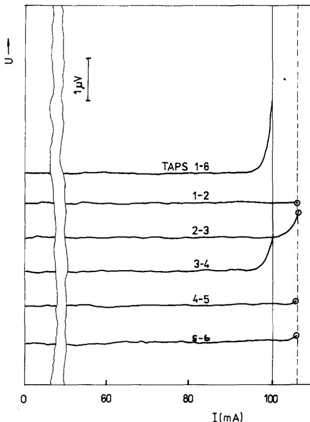
Figure 7 Current–voltage characteristics of the Nb–Ti filament measured between potential taps 1 and 2, 2 and 3, 3 and 4, 4 and 5, 5 and 6 and 1 and 6 (whole sample length) in magnetic field *B* = 5.46 T
