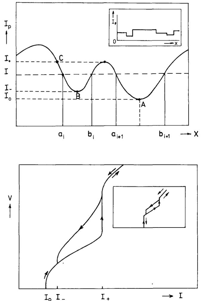
Figure 3 (a) Graphical solution of the equation  $I = I_p(x)$ . The regions  $a_i < x < b_i$  and  $a_{i+1} < x < b_{i+1}$ , where  $I > I_p(x)$ , are in the normal state. Insert, special case: rectangular inhomogeneities. (b) Current-voltage characteristics corresponding to a filament with minimum propagating current distribution shown in (a). Insert, current-voltage characteristic for rectangular inhomogeneities
