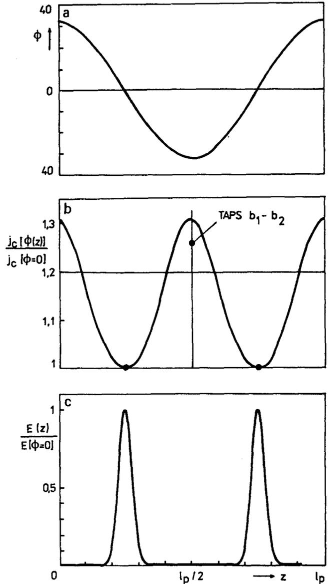
**Figure 8** Variation of: (a)  $\phi$ ; (b)  $j_c[\phi(z)] / j_c[\phi=0]$ ; (c)  $E(z) / E[\phi=0]$  along spiral sample 3 for  $\alpha = 0$  (magnetic field perpendicular to the spiral axis)
