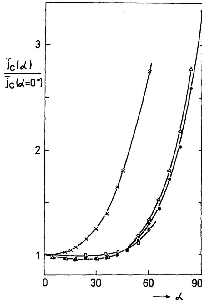
**Figure 7** Angular dependence of ratio  $\tilde{j}_c(\alpha)/\tilde{j}_c(\alpha=0^\circ)$  for spiral sample 3 at: ●, 4.07 and Δ, 3.01 T (measured); and D, 4 T (theory). ×, This curve represents the ratio  $j_c(\phi)/j_c(0)$  for the straight sample as a function of angle  $\phi$
