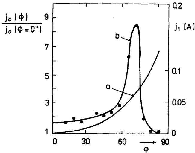
Figure 1 Measured dependence of: (a)  $j_c(\phi)/j_c(\phi=0^\circ)$ ; (b)  $j_l$  on angle  $\phi$ , for  $B=4$  T
