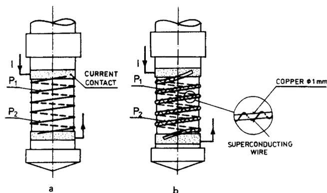
Figure 4 (a) Sample 1 in perpendicular field and (b) spiral sample 2 in a field perpendicular to the spiral axis. Angle  $\zeta$  for the spiral sample is  $\approx 61^\circ$
