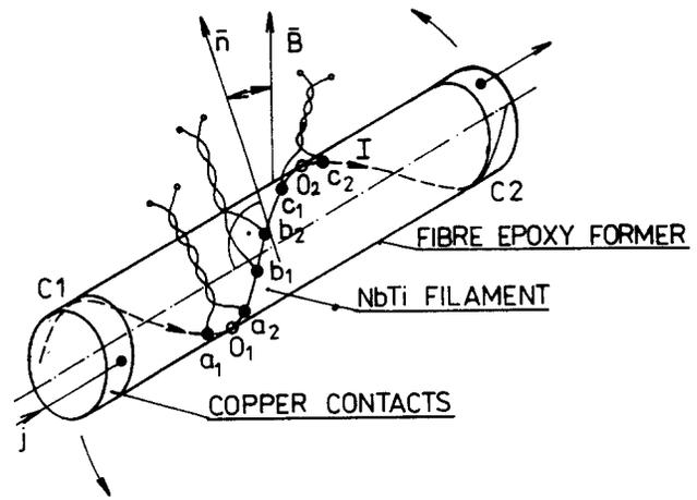
Figure 5 Position of the potential taps on spiral sample 3
