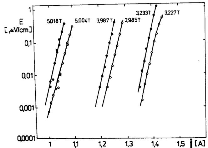
Figure 6 Measured  $E$ - $j$  characteristics of: ●, the straight sample; and ○, sample 2 in fields of  $\approx 5.4$  and 3 T
