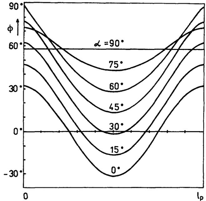
Figure 3 Dependence,  $\phi(z)$ , for the spiral with  $l_p/R = 10$  and different angles of  $\alpha$
