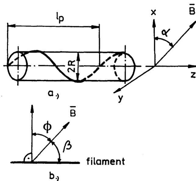
Figure 2 Orientation of the spiral sample and the filament in the co-ordinate system
