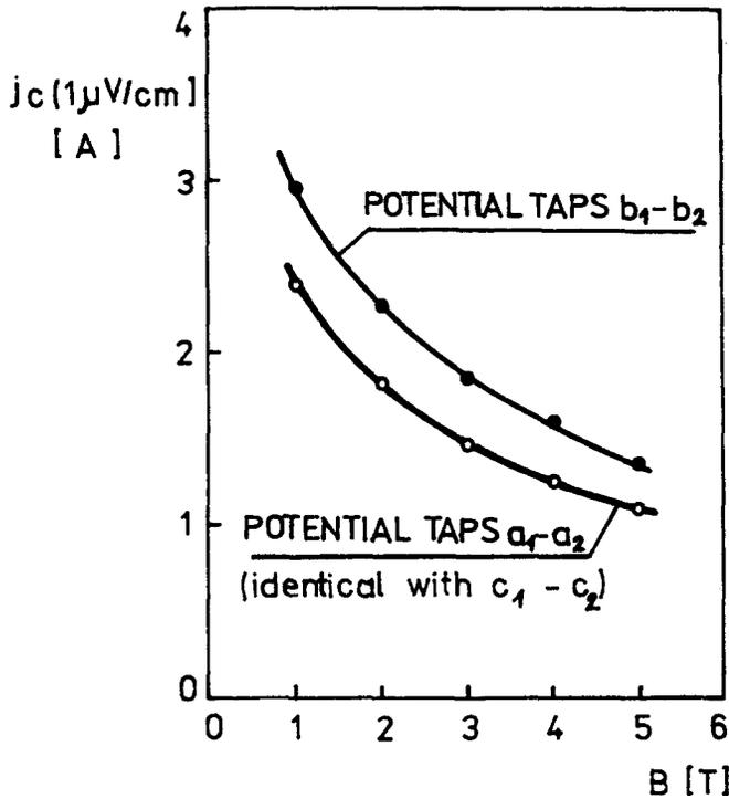
**Figure 9** Critical current,  $j_c$ , for  $E_0=1 \mu\text{V cm}^{-1}$  measured between the potential taps  $a_1$ - $a_2$  and  $b_1$ - $b_2$  on the spiral sample as a function of  $B$ . Values of  $j_c$  between  $a_1$ - $a_2$  and  $c_1$ - $c_2$  are identical
