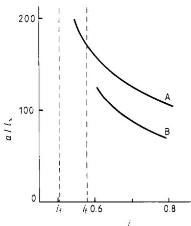
**Figure 10.** Function  $a = a(i)$  for a TRC with parameters: A,  $l_n/l_s = 50$ ,  $l_i/l_s = 100$  and  $h = 0.05$ ; B,  $l_n/l_s = 33$ ,  $l_i/l_s = 75$  and  $h = 0.2$ .
