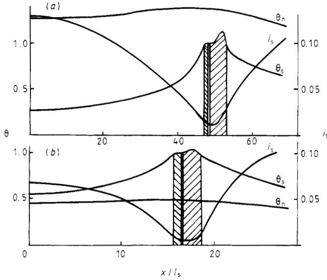
**Figure 5.** Distributions of temperature and current density  $i_s$  at the moment of splitting of a resistive domain: (a) in a TRC with parameters  $l_n/l_s = 33$ ,  $l_i/l_s = 75$  and  $h = 0.2$  for  $i = 0.70$ ; (b) in a FRC with parameters  $l_n/l_s = l_i/l_s = 33$  and  $h = 0.2$  for  $i = 0.50$ .
