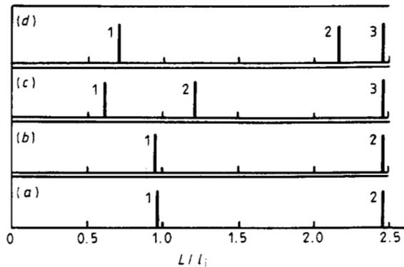
**Figure 12.** Schematic arrangement of resistive domains at different values of the transport current density  $i$ .
