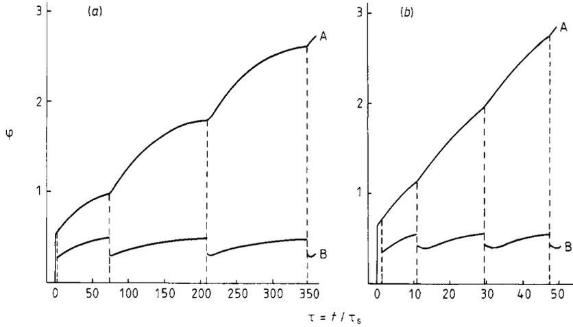
**Figure 8.** Functions  $\varphi = \varphi(t)$  (A) and  $\varphi' = \varphi'(t)$  (B) for a TRC with parameters  $l_n/l_s = 50$ ,  $l_i/l_s = 100$  and  $h = 0.05$  for (a)  $i = 0.55$  and (b)  $i = 0.70$ .
