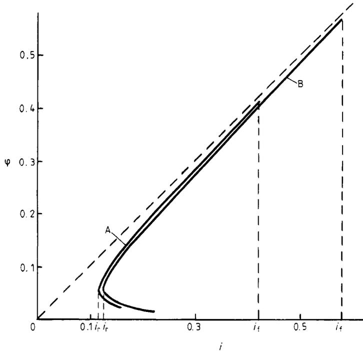
**Figure 3.** Current-voltage characteristics: A, for a FRC with parameters  $l_n/l_s = \bar{l}_1/\bar{l}_s = 33$  and  $h = 0.2$ ; B, for a TRC with parameters  $l_n/l_s = 33$ ,  $l_1/l_s = 75$  and  $h = 0.2$ .
