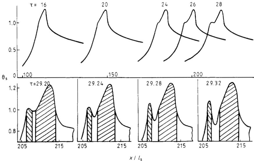
**Figure 6.** Evolution of temperature distribution in the superconducting component during the splitting of the resistive domain in a TRC with parameters  $l_n/l_s = 50$ ,  $l_i/l_s = 100$  and  $h = 0.05$  for  $i = 0.70$ .
