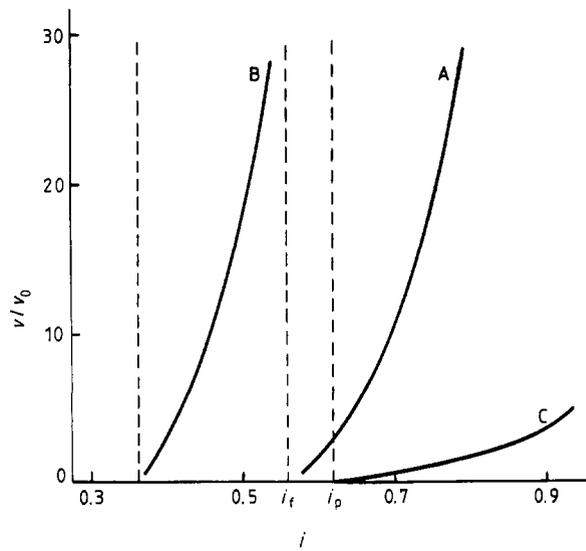
**Figure 9.** Functions  $v = v(i)$ : A, for a TRC with parameters  $l_n/l_s = 33$ ,  $l_i/l_s = 75$  and  $h = 0.2$ ; B, for a FRC with parameters  $l_n/l_s = \bar{l}_i/\bar{l}_s = 33$  and  $h = 0.2$ ; C, for a composite equivalent to the TRC and the FRC with zero contact resistance.
