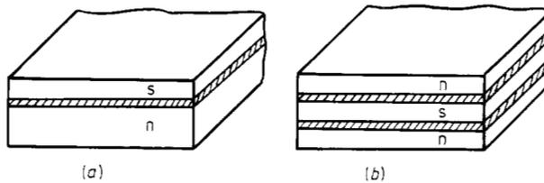
Figure 1. Specimen geometry. The shaded area indicates the transition layer. (a) TRC and (b) FRC.
