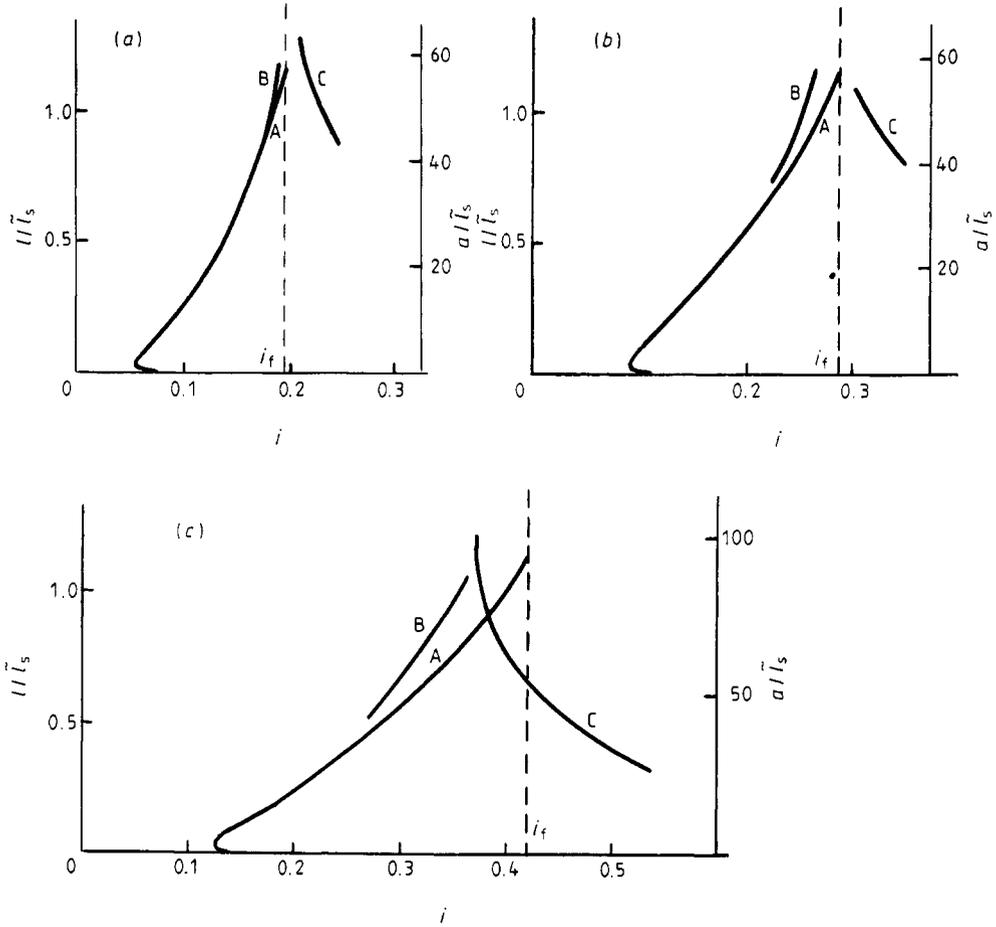
**Figure 2.** Curves  $l = l(i)$  and  $a = a(i)$  for the FRC with parameters  $l_n/l_s = \bar{l}_i/\bar{l}_s = 33$ .  $l = l(i)$ ; A,  $\theta_n = 0$ ; B,  $\theta_n$  is allowed to rise; C,  $a = a(i)$ . (a)  $h = 0.05$ , (b)  $h = 0.1$ , (c)  $h = 0.2$ .
