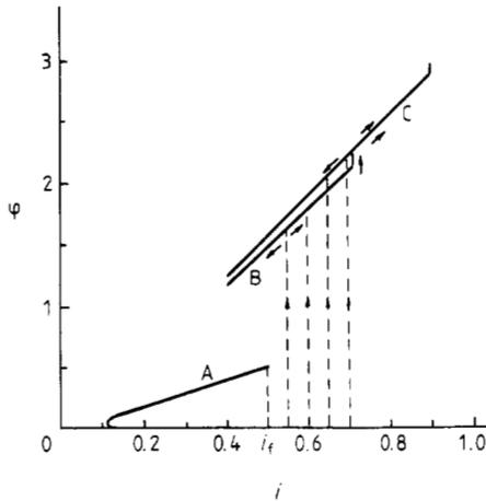
**Figure 11.** Current-voltage characteristic of a specimen with resistive domains (a TRC with parameters  $l_n/l_s = 50$ ,  $l_i/l_s = 100$  and  $h = 0.05$ ). The specimen contains a single domain (A), four domains (B) and six domains (C).
