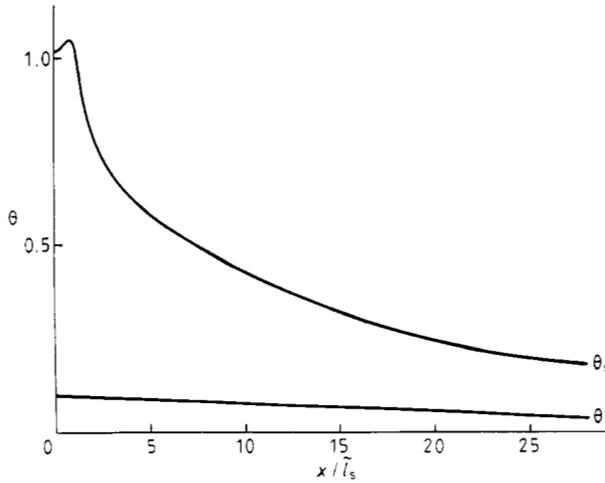
Figure 4. Steady-state temperature distributions in the normal and superconducting components of a FRC with parameters  $l_n/l_s = \bar{l}_i/\bar{l}_s = 33$  and  $h = 0.05$  for  $i = 0.19$ ,  $i_f = 0.2$ .
