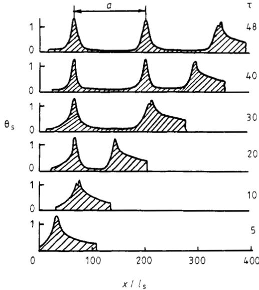
Figure 7. The process of formation of a string of resistive domains in a TRG with parameters  $l_n/l_s = 50$ ,  $l_i/l_s = 100$  and  $h = 0.05$  for  $i = 0.70$ .
