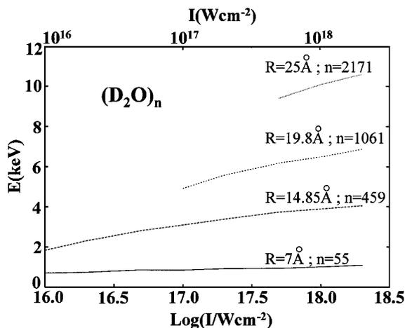
FIG. 3. Simulations of Coulomb explosion of  $(D_2O)_n$  clusters, showing the dependence of the maximal  $D^+$  energies on the laser intensity. Cluster sizes are marked on the curves.
