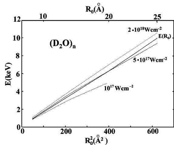
FIG. 4. The dependence of the  $D^+$  maximal energy from the Coulomb explosion  $(D_2O)_n$  clusters on  $R_0^2$ . The numbers on the dashed curves represent the laser intensities. The solid line represents  $E(R_0)$ , Eq. (2).
