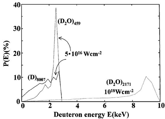
FIG. 5. The deuteron energy distribution in the Coulomb explosion of  $(D_2O)_n$  ( $n = 450, 2171$ ) and  $(D)_n$  ( $n = 8007$ ) clusters.  $P(E)$  is presented as percents per the energy interval of 0.2 keV. The numbers on the curves represent the laser intensity.
