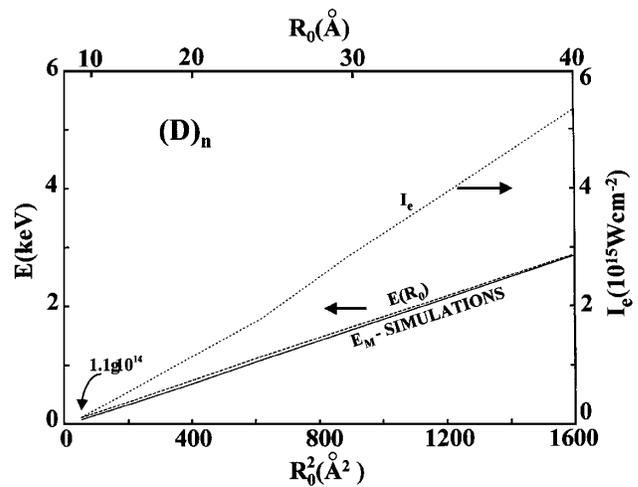
FIG. 2. The cluster size dependence of the  $D^+$  energies at the saturation level ( $E_M$ ) and the saturation intensities ( $I_e$ ) from simulations of the Coulomb explosion of  $(D)_n$  clusters. Also given is the CSE for  $E(R_0)$ , Eq. (1).
