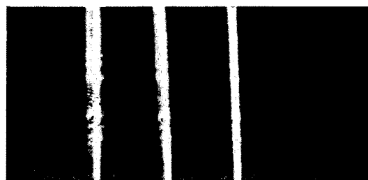
Fig. 2. The distribution of the incident light within the crystal. The photographs show the intensity distribution for a slab, with the laser light passed through the optical system, and emerging through a 0.3-mm-thick anthracene crystal. The thickness of the slab (from left to right): D_0=24 \mu , D_0=24 \mu , D_0=34 \mu , and D_0=48 \mu .
