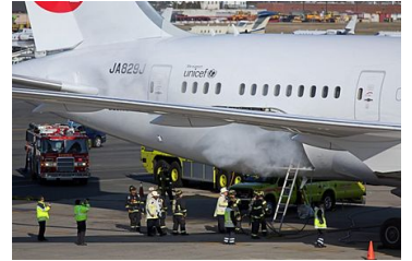
Japan Airlines 787 Dreamliner at Boston Logan Airport with lithium-ion battery fire and resulting heavy smoke coming out a cargo hold
