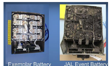
Japan Airlines 787 battery comparison; Left: typical original battery. Right: damaged battery.
