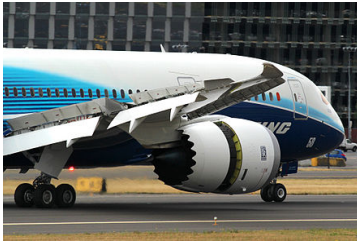
The chevron-toothed exhaust duct covers on the first 787, shown here with thrust-reversers deployed
