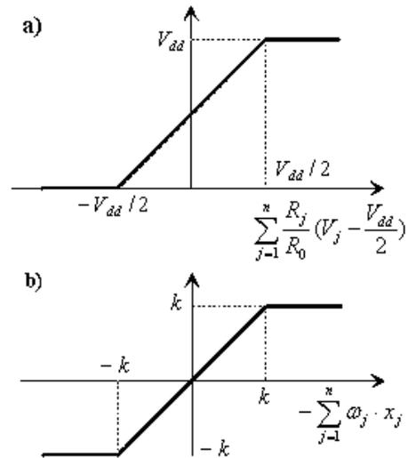
**Figure 2.** Summing amplifier's behavior representation: within voltage coordinates (a); within multi-valued variables coordinates (b).
