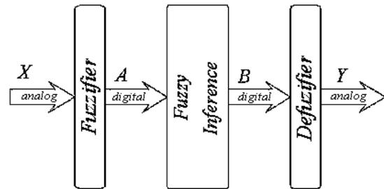
**Figure 5.** Fuzzy device structure.
