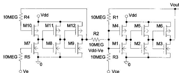
**Figure 7.** CMOS implementation of the fuzzy controller, specified by Tab.2.
