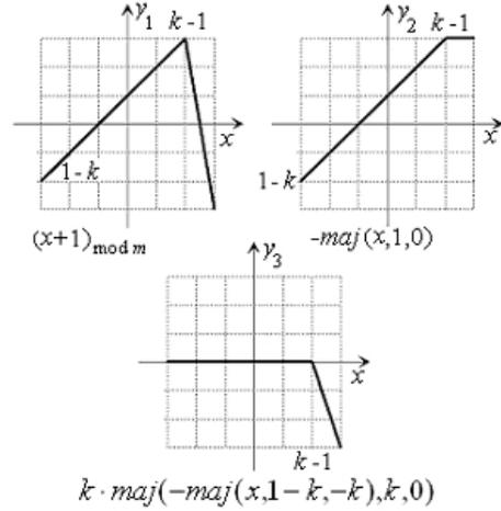
**Figure 4.** Implementation of  $(x+1)_{\text{mod } m}$  function.
