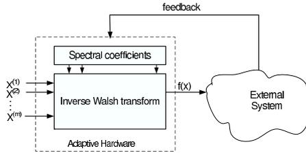
Figure 1: The architecture of a WbAH system
