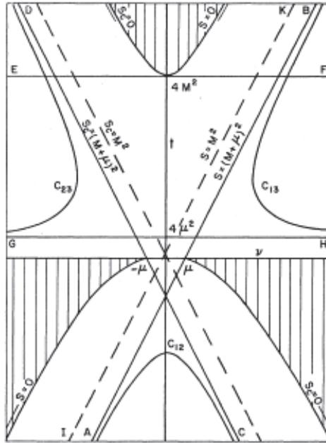
Fig. 1. The Mandelstam plot for  $\pi N$  scattering, taken from the original paper.<sup>1</sup> Masses of  $\pi$  and  $N$  are denoted by  $\mu$  and  $M$ , respectively. The physical region of  $s$  is the shaded region on the bottom right.
