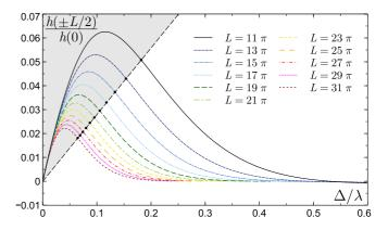
FIG. 8. (Color online) Evolution of the normalized height of the exact solution (A6a) at the boundaries as a function of the normalized displacement. The dots indicate the position of the threshold,  $\Delta_F/\lambda$ , below which the profile is periodic. The shaded area corresponds thus to the wrinkle state. This area is delimited by the relation  $h(\pm L/2)/h(0) = 0.279 \, \Delta_F/\lambda = 0.279 \, \lambda/L$ .
