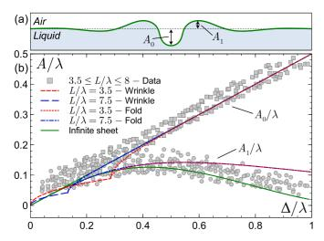
FIG. 7. (Color online) (a) Definitions of the amplitudes  $A_0$  and  $A_1$  for the localized state. (b) Comparison between the experimental evolution of  $A_0$  and  $A_1$  (rescaled by  $\lambda$ ) with increasing confinement for finite sheets [42], and the prediction of Eq. (45b) where  $A_0 = |h(0)|$  and  $A_1 = |h(\pi)|$ . The evolution of the amplitudes of the exact solution for an infinite sheet is also presented [45].
