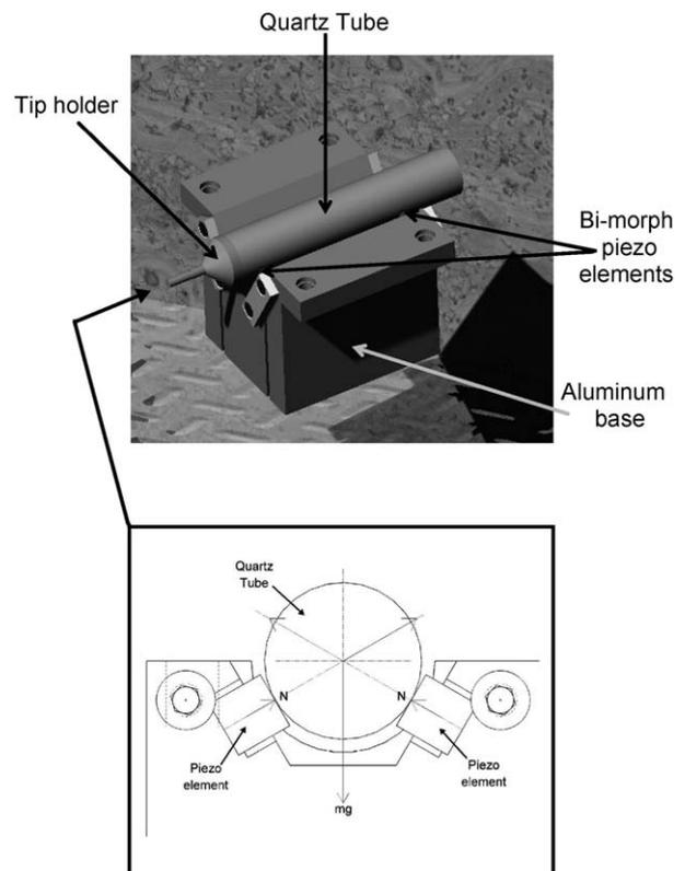
Fig. 4. The general description of a linear piezo-stepper motor made of four legs of bi-morph piezo elements and quartz tube.
