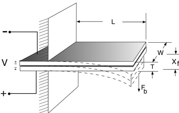
Fig. 3. The cantilever configurations of bi-morph element.
