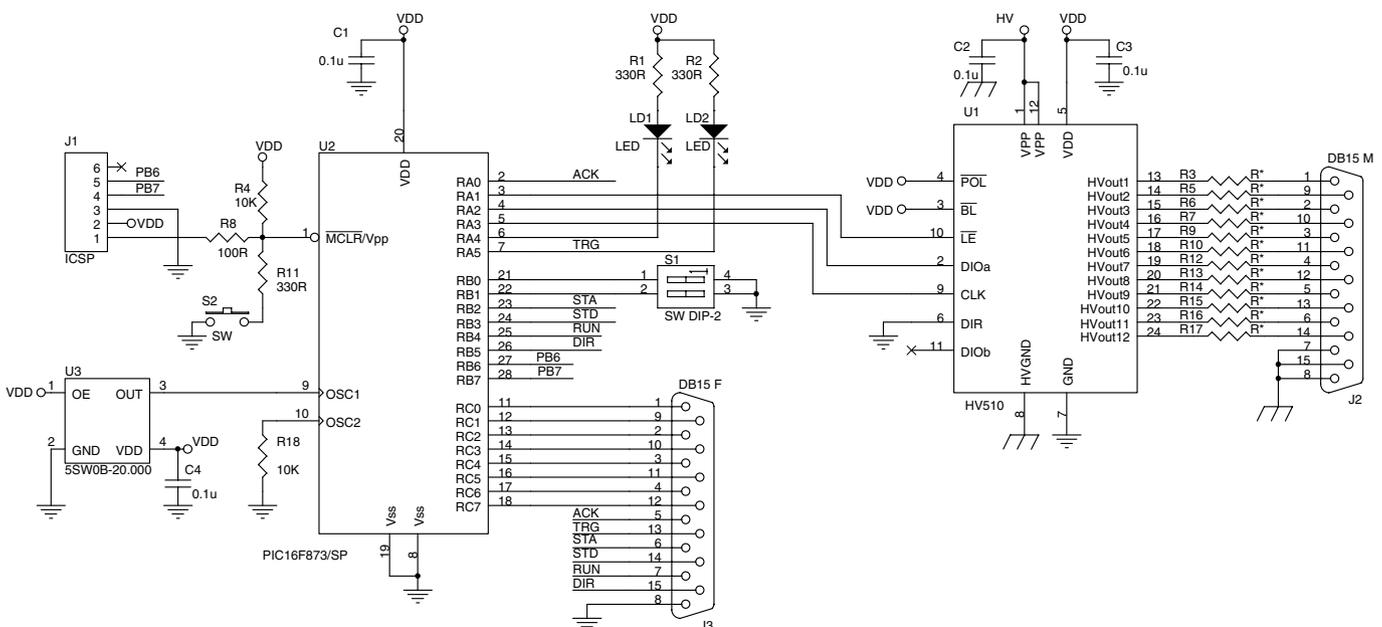
Fig. 1. The controller circuit diagram. U<sub>1</sub> is HVC MOS device that receives 12 data bits serially by DIO and CLK inputs and sends the converted high-voltage signal in parallel through J<sub>2</sub>. The data and timing signals are controlled by U<sub>2</sub>—PIC16F873 microcontroller.
