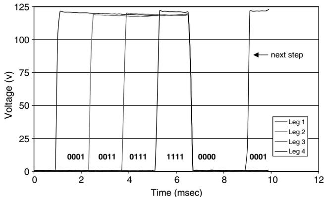
Fig. 5. The voltage waveform that is used for the piezo-stepper motor. The string length is 5 and the sequential pulses for a forward step are  $\{(0001), (0011), (0111), (1111), (0000)\}$  where the 0 and 1 represent 0 V and 120 V on each leg. The internal delay is 1500  $\mu\text{s}$  while the external delay is 8 ms.
