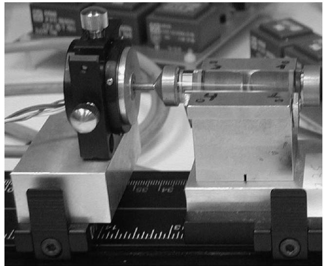
Fig. 7. The overall system: the quartz tube, which carries the tip, the aluminum base with the four bi-morph elements, and the LVDT that measures the step size.
