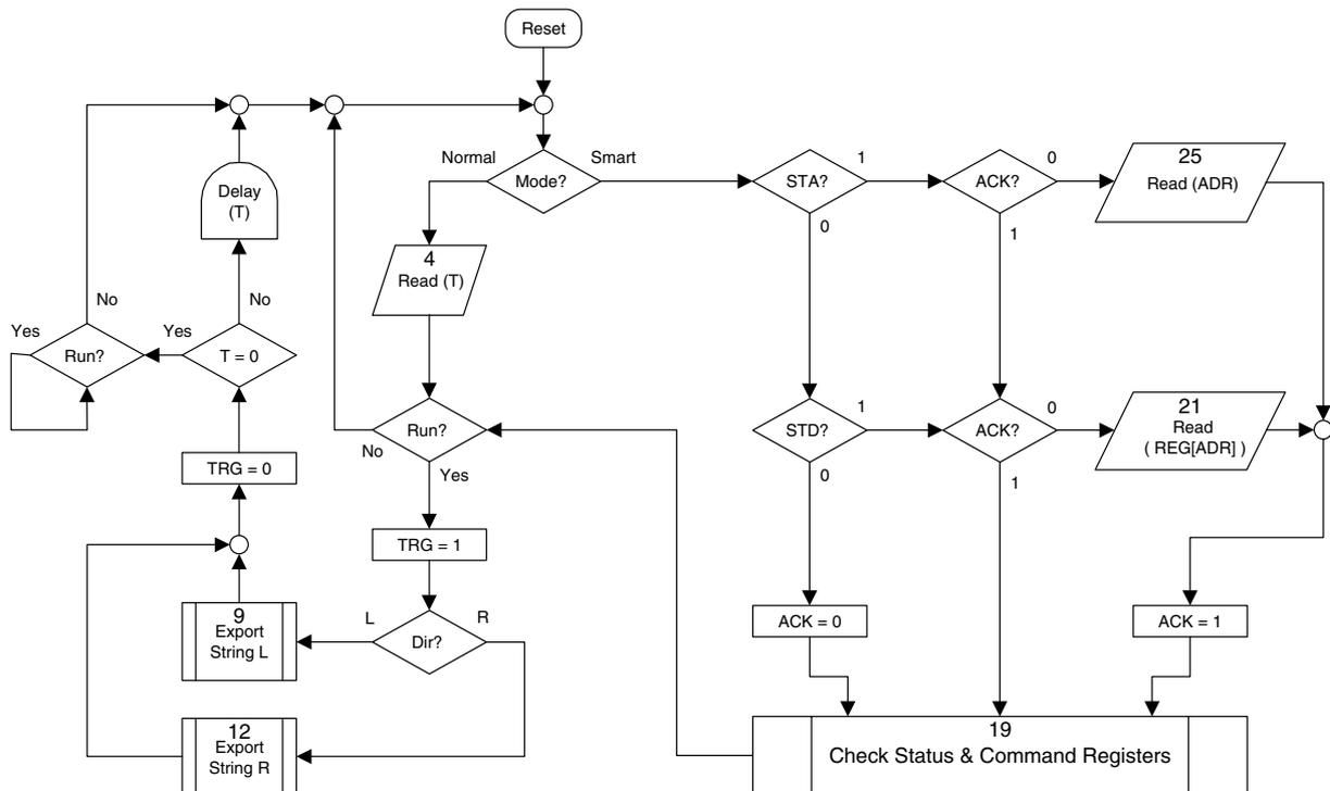
Fig. 2. The flowchart of the controller embedded program for normal and smart modes.
