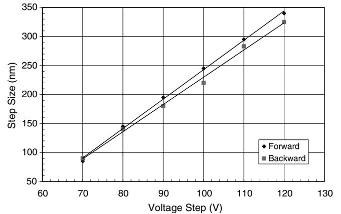
Fig. 6. The step size as a function of the voltage (measure by LVDT).
