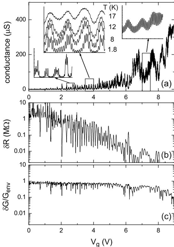
FIG. 1. (a) Conductance as a function of gate voltage measured at  $T = 1.8$  K. Some regions are enlarged in the insets. In (b) and (c) the amplitude of the fast oscillations is extracted from the curve in (a) in units of resistance  $\delta R$  and in units of conductance, normalized by the envelope of the total conductance,  $\delta G/G_{\text{env}}$ .
