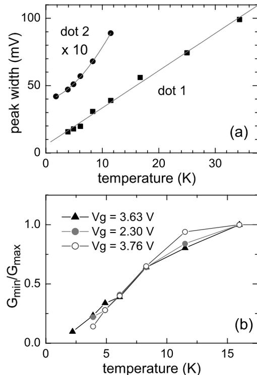
FIG. 4. (a) Scaling of the peak full width at half maximum (FWHM) with temperature is plotted for both dots. The lines are the linear and parabolic fits for dot 1 and dot 2, respectively. Peak width for dot 2 is multiplied by a factor of 10 for visibility. The peaks are close to  $V_g = 3$  V. (b) Temperature dependence of the peak-to-valley ratio for the fast oscillations. Solid (open) symbols are for the ratios taken near the peaks (valleys) of the slow oscillations.
