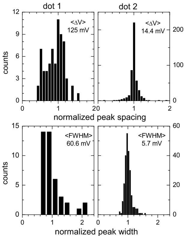
FIG. 3. Histograms of peak spacing (top) and width (bottom) are plotted for dot 1 (left) and dot 2 (right).
