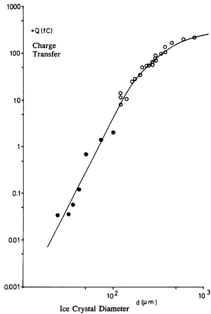
the *relative* diffusional growth rates of the interacting ice particle surfaces was the factor that controls the sign of charge transfer. The charge transfer follows the rule that the ice surface that grows faster by vapour diffusion charges positively during ice crystal/graupel
