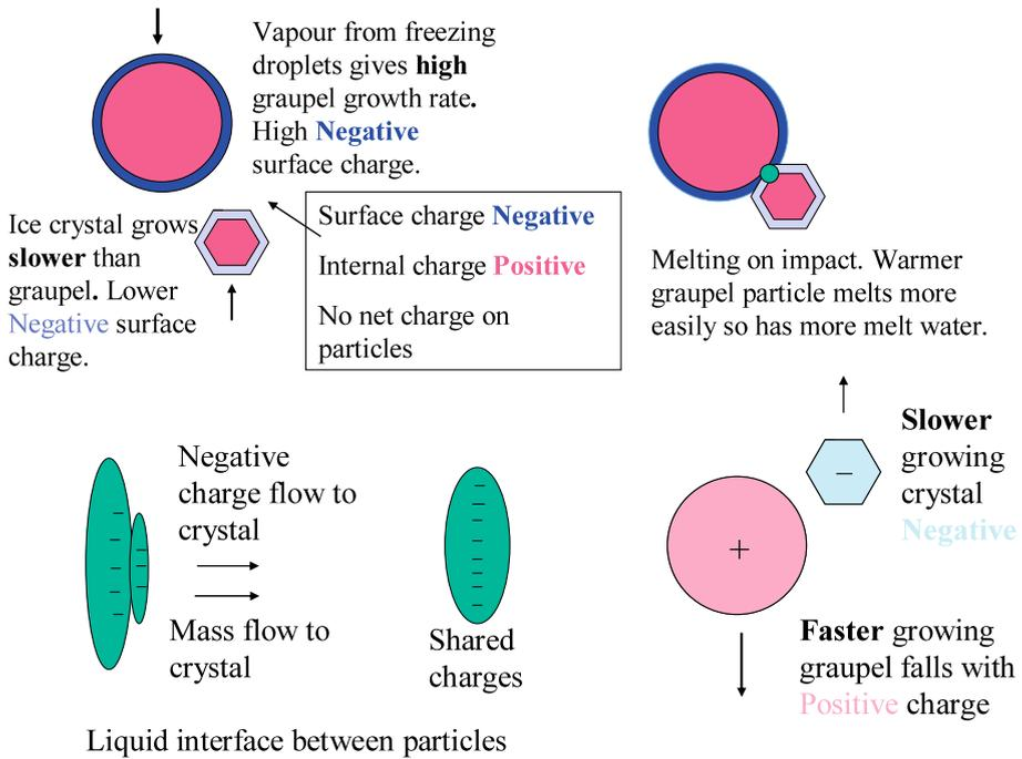
**Fig. 11** A graupel pellet, warmed by rime accretion collides with a colder, faster growing, ice crystal. Charges and mass are shared in the melt water. The graupel becomes negatively charged while the crystal carries positive charge
