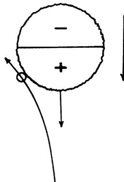
**Fig. 3** Collisions between nearly equal sized water drops result in particle separations in the direction of the vertical environmental electric field that are in a direction to dissipate the field. (Al-Said 1977)
