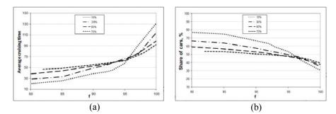
Fig. 7.5 (a) Average cruising time ( $T_{cruising}$ ) in seconds; and (b) Share of cars parking without cruising (P<sub>0</sub>) for average turnover rates of 15%, 30%, 50%, and 70%.
