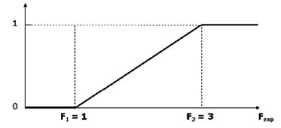
**Fig. 7.3** The probability to continue driving when passing a free parking place as a function of the expected number of free parking places between driver's location and destination (Benenson et al., 2008).
