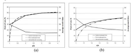
Fig. 7.8 Share of cars parking without cruising ( $P_0$ ) and average search time ( $T_{\text{search}}$ ): (a) e = 1,000 cars/hour,  $a = 1,000 \div 4000 \text{ cars/hour}$ , (b) e = 5,000,  $a = 5,000 \div 8,000 \text{ cars/hour}$ .
