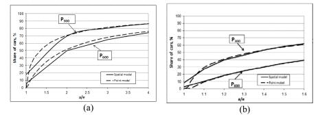
Fig. 7.9 Share of cars that search for parking longer than 300 and 600 seconds ( $P_{300}$  and  $P_{600}$ ): (a) e = 1000 cars/hour,  $a = 1000 \div 4000$  cars/hour, (b) e = 5,000,  $a = 5000 \div 8000$  cars/hour.
