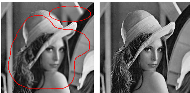
Fig. 3. Non-blind space-variant restoration with different blur kernels in each region. Left: Blurred image. Right: Restoration using the suggested method.
