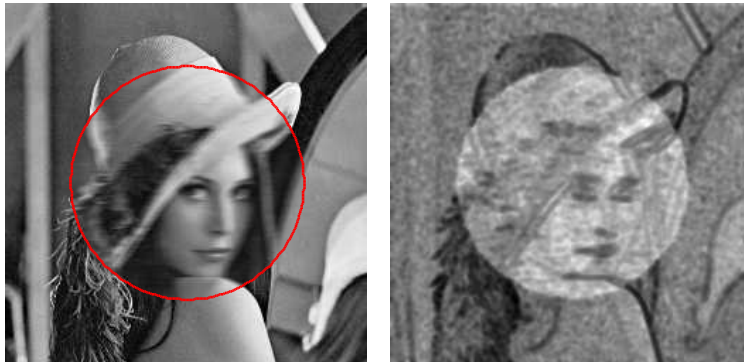
Fig. 4. Left: Blurred image. Right: The corresponding E function.
