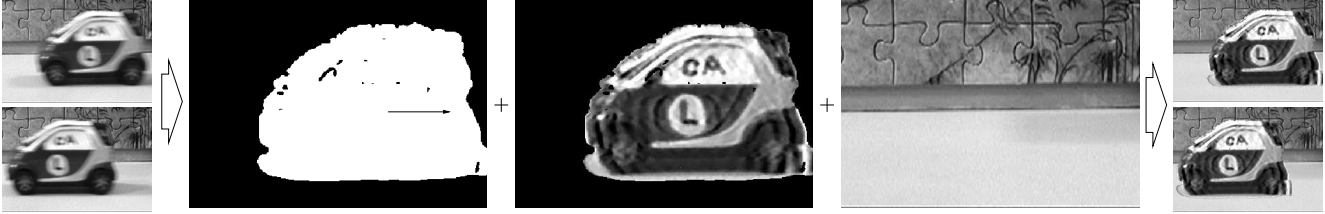
Figure 1. From two real blurred frames (left), we automatically and simultaneously estimate the motion region, the motion vector, and the image intensity of the foreground (middle). Based on this and the background intensity we reconstruct the two frames (right).
