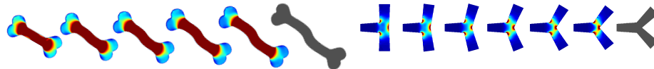
Fig. 4. Discrete geodesic for two different examples from [2] and [23] where the local rate of dissipation is color-coded as . In the right example the local preservation of isometries is clearly visible, whereas in the left example stretching is the major effect.
