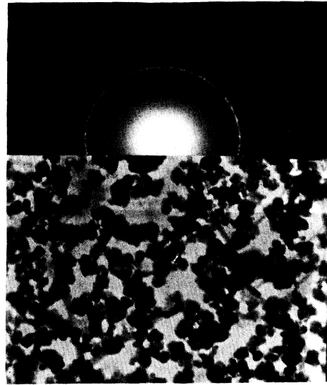
FIG. 4. The bright field and diffraction pattern of the Ge after the Al was etched out.
