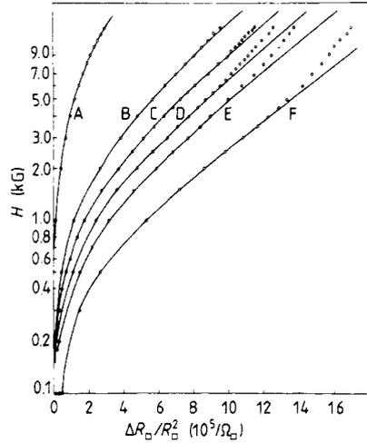
**Figure 3.** Semi-log plot of the perpendicular-field MR for all the samples. The full curves were fitted.  $H_{c_2}^*$  is the field where the curve stops fitting the data.
