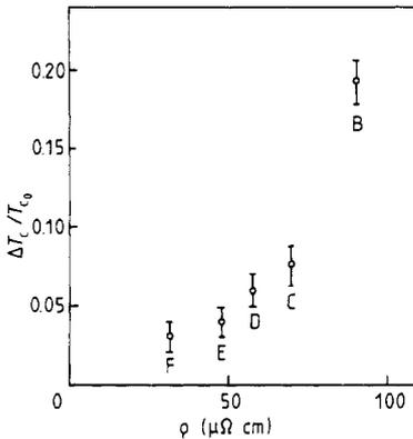
Figure 6. The variation of the superconducting transition temperature with the normal-state resistivity.
