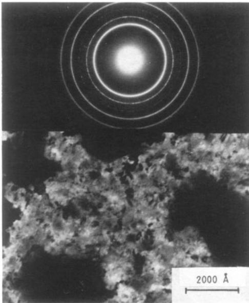
**Figure 1.** A TEM micrograph and diffraction pattern for In-Ge (the sharp circles are for Ge and the dotted ones for In).
