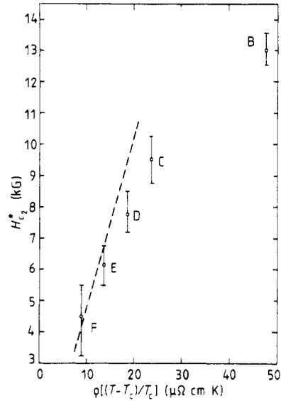
Figure 5.  $H_{c2}^*$ , the critical field where the deviation from the fitted curve starts, versus the sample resistivity. The broken line is drawn with the slope that intersects the pure In parameters ( $T_c = 3.4$  K and  $H_{c2}^* = 300$  G).
