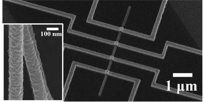
FIG. 1. A SEM image of a typical nanowire connected to Ohmic contacts. The dark area surrounding the nanowire is the hardened PMMA. The inset shows typical superconducting coated nanowires with  $d = 100$  nm.
