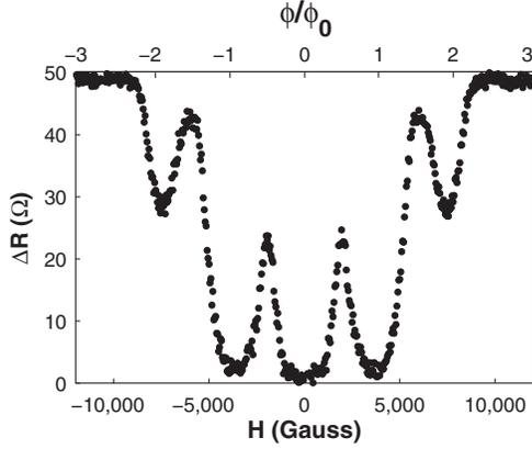
FIG. 3. The residual resistance as a function of magnetic field (bottom axis) and flux (top axis) of sample b4. The diameter of the cylinder is estimated to be 83 nm, and the zero temperature coherence length 79 nm.
