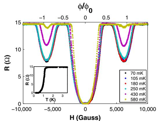
FIG. 2 (color online). Resistance as a function of magnetic field of sample e7 at several temperatures. The diameter of the cylinder is estimated to be 66 nm, and the zero temperature coherence length 110 nm. The inset shows the transition of sample e7 into the superconducting phase.
