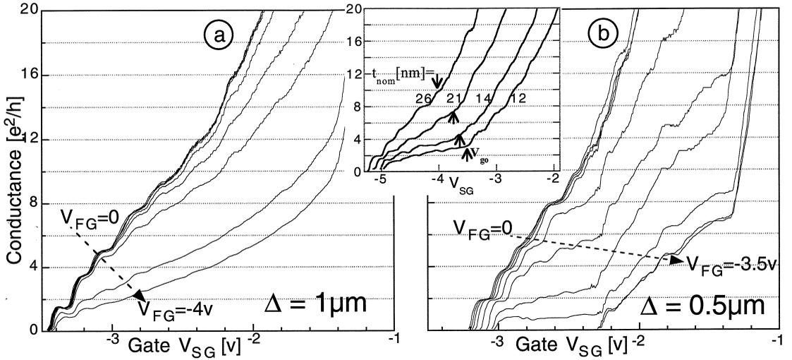
Fig. 2. Conductance versus straight-gate voltage measured for the sample with nominal QW thickness of 26 nm at 4.2 K while the fork-shaped-gate voltage is the tuning parameter (mostly in steps of 0.5 V). The QWR “access” length  $\Delta$  is 1  $\mu\text{m}$  in (a) and 0.5  $\mu\text{m}$  in (b). In the inset, the conductance is plotted for structures different nominal QW thickness (12, 14, 21 and 26 nm).
