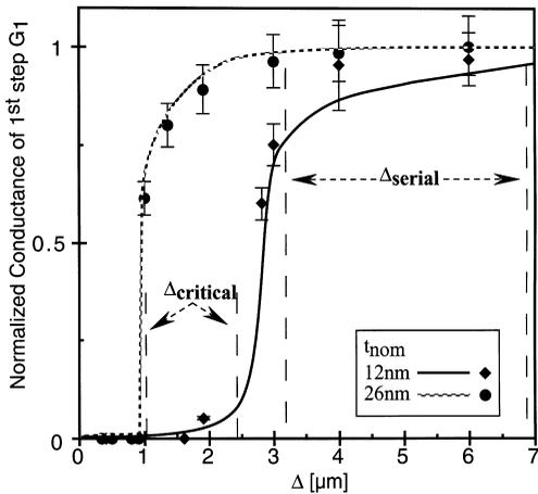
Fig. 3. The normalized conductance of the first step versus the QWR “access” length  $D$ , for structures with different QW nominal thickness (12 and 26 nm) corresponding to different strength of 1D confinement (symbols). The curves serve as a guide-to-the-eye to clarify the characteristic lengths  $\Delta_{\text{critical}}$  and  $\Delta_{\text{serial}}$ .
