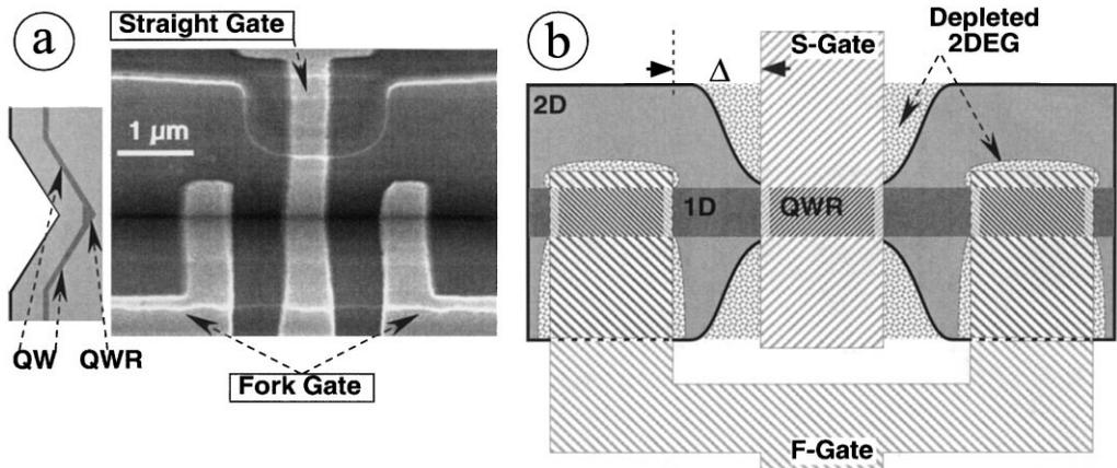
Fig. 1. (a) SEM image of an isolated single V-groove top-gated by the two independent gates. (b) A schematic illustration showing the QWR definition by the straight gate and the access length  $\Delta$  defined by the fork-shaped gate. The QWR is connected to two electron reservoirs in which the conductance proceeds in parallel in 2D and 1D regions.
