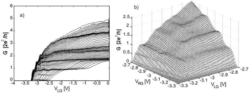
Fig. 4 – a) Conductance (in units of  $2e^2/h$ ) of the device in fig. 3b) *vs.* gate LG voltage, with gate RG voltage as parameter (curves from top to bottom correspond to  $V_{RG}$  varying from  $-2.7$  V to  $-3.3$  V at  $0.01$  V intervals). b) Conductance (in units of  $2e^2/h$ ) of the device in fig. 3b) *vs.* the voltage on both gates (varying from  $-2.7$  V to  $-3.3$  V at  $0.01$  V intervals).
