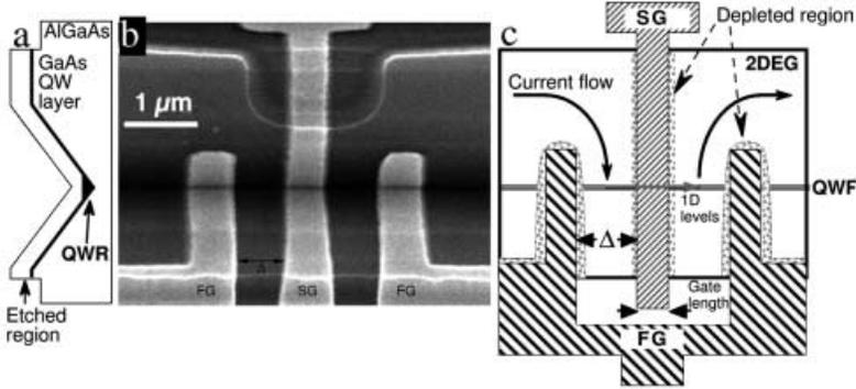
Fig. 1 – a) Schematic cross-section of a QWR device. b) Scanning electron micrograph (top view) of a device with a straight gate SG and a fork gate FG at an inter-gate distance  $\Delta$ . c) Schematic diagram of the device, showing the current path and depleted regions.
