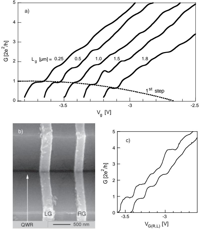
Fig. 3 – a) Conductance (in units of  $2e^2/h$ ) of QWR sections of lengths 0.25–1.8  $\mu\text{m}$ , as defined by the length of a single gate (similar to SG in fig. 1). The line connecting the first plateaus is a guide to the eye. b) Scanning electron micrograph (top view) of a device with two straight gates, RG (right) and LG (left). c) Conductance (same units) of the device in fig. 1a) *vs.* voltage of each of the two gates, while the other gate is maintained at 0 V.
