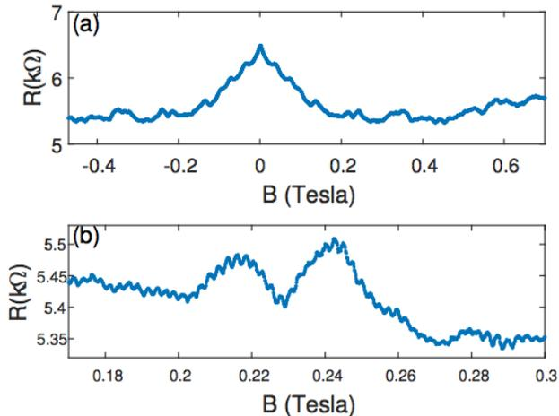
FIG. 5. (Color online) (a): The magnetoresistance of an Aharonov-Bohm ring at 1.5 K, as a function of the magnetic field, up to  $B = 0.7$  Tesla. (b) The magnified data in the low-field region, showing the tiny oscillations superimposed on the Aharonov-Bohm ones.
