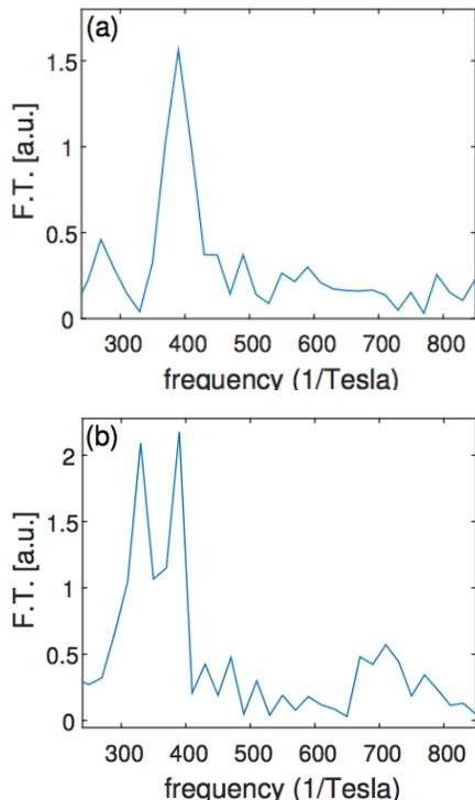
FIG. 7. (Color online) (a) The Fourier transform of the magnetoconductance for magnetic fields in the range 0.1–0.15 Tesla; the main peak is at  $\approx 390 \text{ Tesla}^{-1}$ . (b) The Fourier transform of the magnetoconductance for magnetic fields in the range 0.65–0.7 Tesla, where the peaks are at  $\approx 330 \text{ Tesla}^{-1}$  and  $\approx 390 \text{ Tesla}^{-1}$ .
