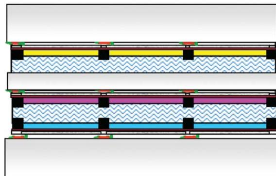
**Fig. 11** A colored electrowetting pixel with layers of oil in different colors (CMY) placed above each other. Adapted with permission from Ref. 19c.
