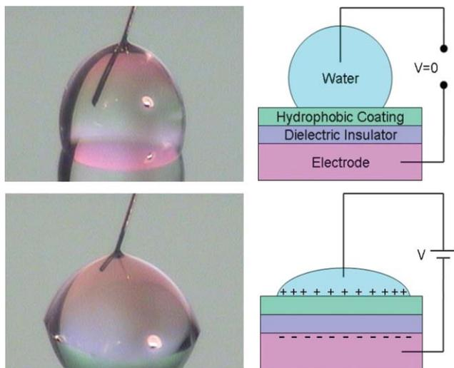
**Fig. 4** Top: A water drop placed on a hydrophobic surface with a high contact angle. Bottom: Electrowetting of the surface. Operation of voltage between the drop and the electrode changes the distribution of charges due to the dielectric insulator and significantly decreases the contact angle. The two surface coatings are drawn not to scale.
