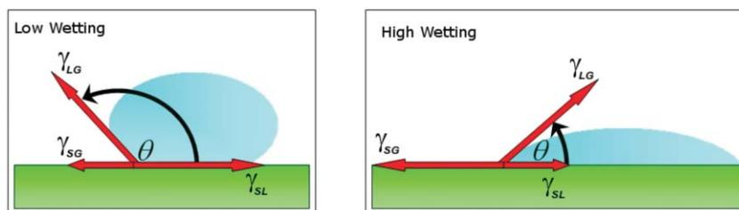
**Fig. 3** Different degrees of wetting. On the left, the wetting is low and the contact angle is large. On the right, the wetting is high and the contact angle is small.
