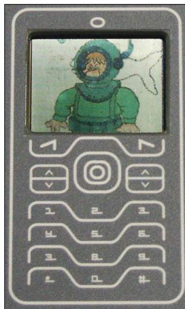
**Fig. 13** An example of a Liquavista Company electrowetting screen in a small electronic device.
