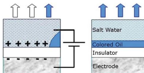
**Fig. 9** Side view of two monochromatic pixel states based on electrowetting. On the right the reflected light is blue (the color of the layer of oil) with no electric voltage, and on the left, with application of the voltage, the light is white (the color of the insulating layer). Adapted with permission from Ref. 19c.
