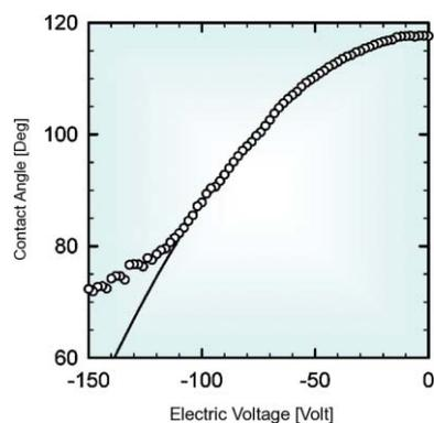
**Fig. 5** Measurement of the contact angle as a function of electric voltage, compared to the theoretical prediction from the Young–Lippmann equation. At voltages lower than  $-110$  volts (depending on the system) the contact angle is saturated, in contradiction to the theoretical prediction. The figure is adapted with permission from Ref. 5.
