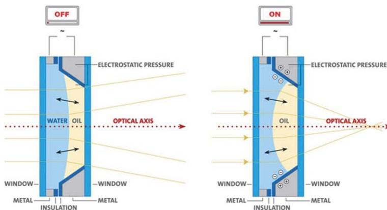
**Fig. 7** Left: A vertical cut through an optical lens consisting of an oil drop in a water medium. Here electric voltage is not turned on and the concave oil drop diffuses the light due to the refractive index of oil which is larger than that of water (Snell's law). Right: Here electric voltage is turned on, and under its influence the water pushes the oil drop to become convex and focus the light passing through it.
