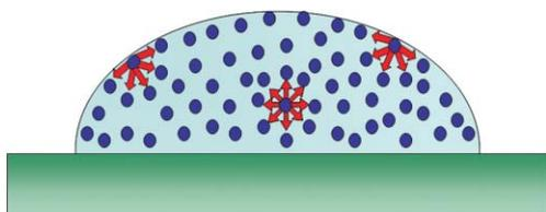
**Fig. 2** The molecules within the drop are equally attracted in all directions, whereas the molecules on the surface of the drop are attracted inward to their neighbors—and that is the source of surface tension.
