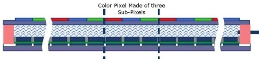
**Fig. 10** A colored electrowetting pixel composed of three monochromatic pixels in the optical primary colors (RGB). Adapted with permission from Ref. 19c.
