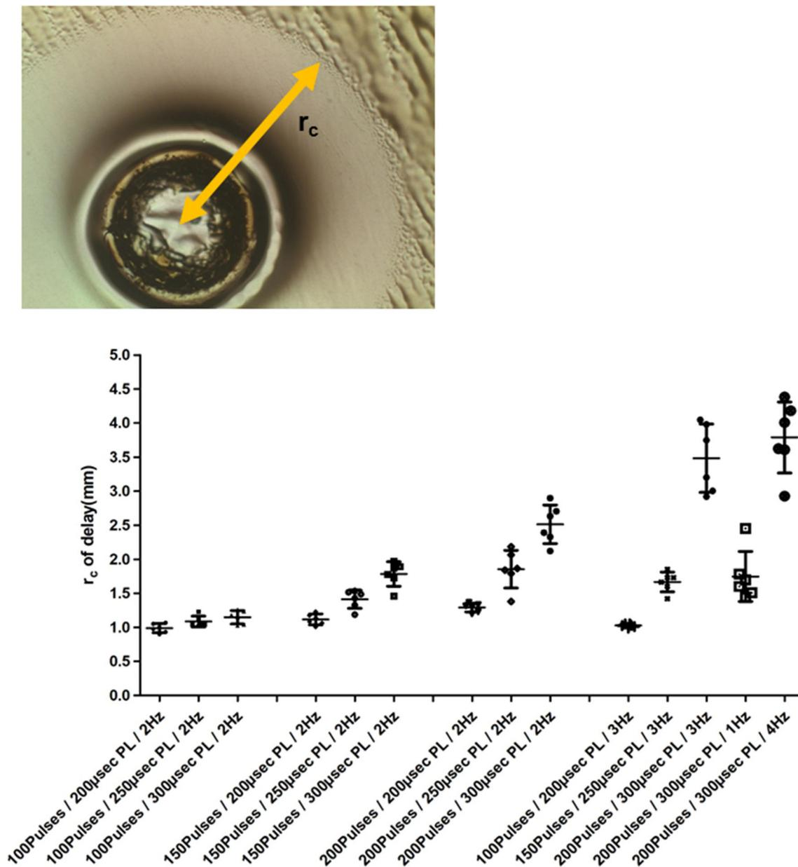
FIGURE 4. Disinfected area by pulsed electric field delivered with a single needle. Top panel: digital image of a sample gel that shows the disinfected area. Bottom panel: The dependence of the disinfected area on the applied pulsed electric field parameters.
