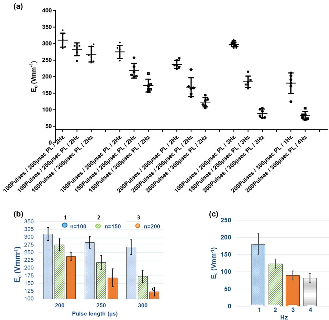
**FIGURE 3.** The threshold of the electric field strength ( $E_c$ ) required for complete inactivation of *Pseudomonas aeruginosa* PAO1. (a) Data from all performed experiments. (b) The dependence of  $E_c$  on the pulse duration. (c) The dependence of  $E_c$  on the frequency of pulse delivery for 200 pulses with 300 μs pulse duration. For each point  $n = 6$ .
