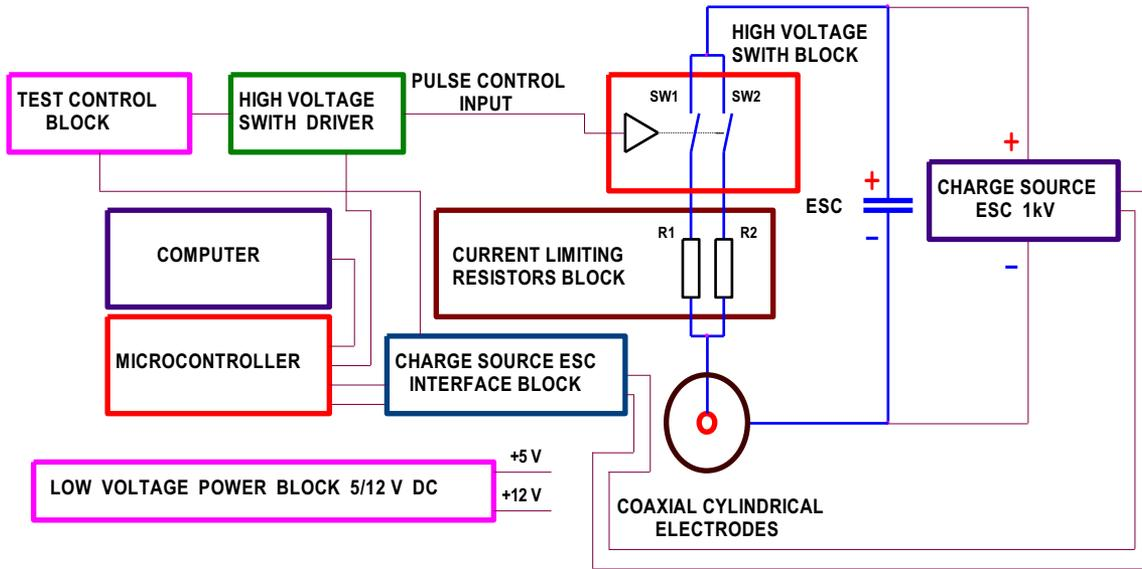
FIGURE 1. Schematic design of the functional units of the pulsed electric field generator.
