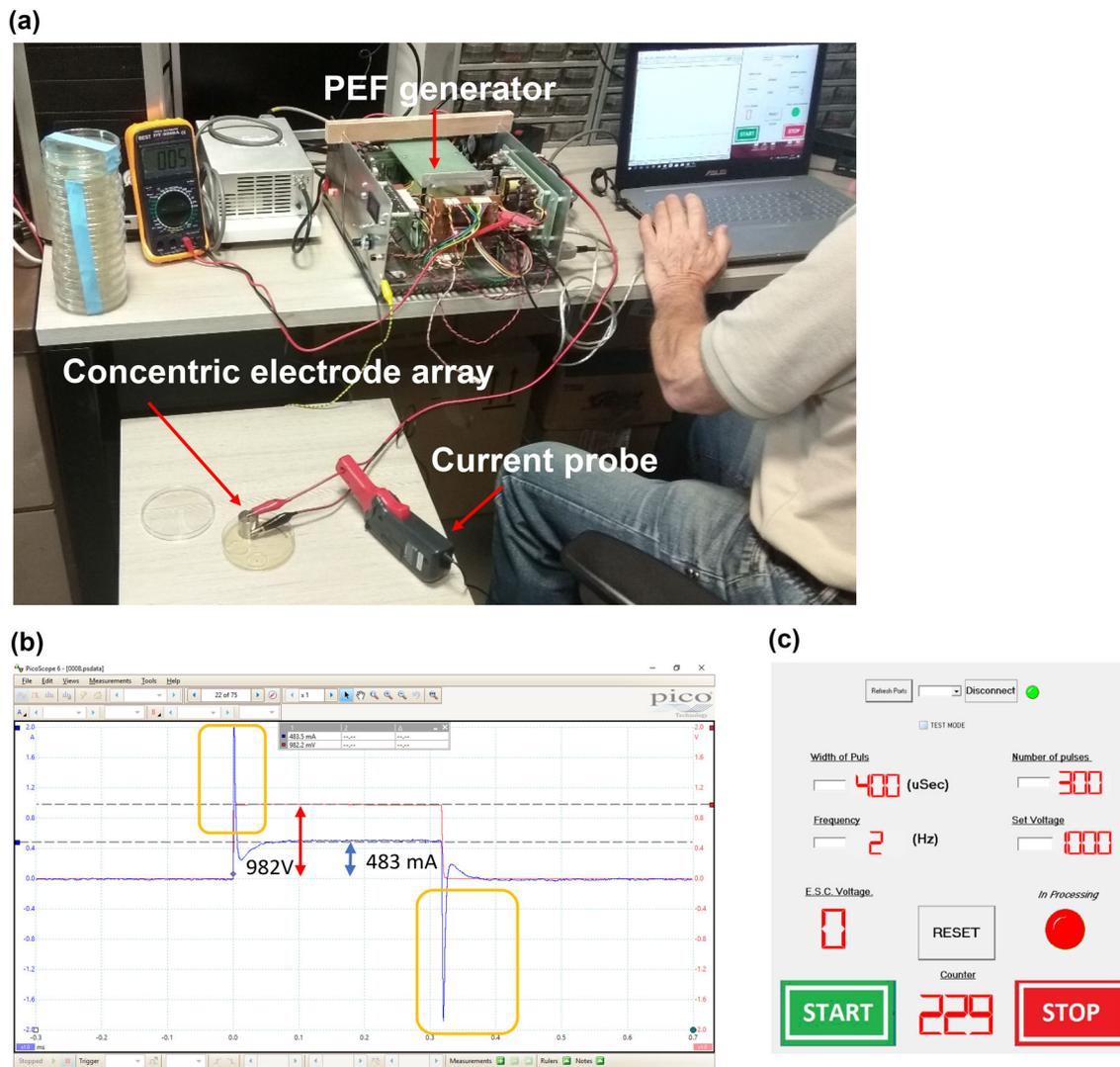
**FIGURE 2.** (a) Digital image of the experimental setup. (b) The current and voltages shape of the single pulse. Spikes, caused by capacitance and inductance are highlighted. (c) Control software screen snapshot.
