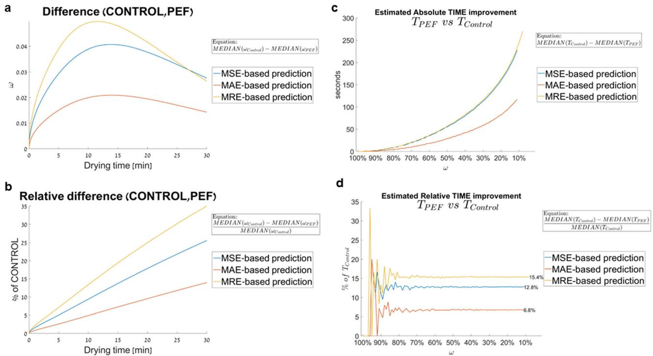
**Fig. 5** **a** Absolute and **b** relative differences between median moisture contents in control and PEF-treated chicken breast muscle in time. **c** Absolute and **d** relative time enhancement of chicken drying expressed
