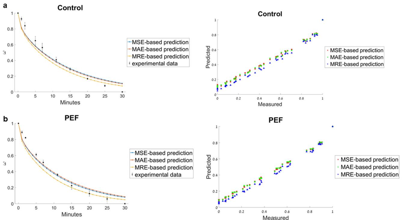
**Fig. 4** Kinetics of the chicken breast drying. Experiment and predicted values based on the mean square error (MSE); the mean absolute error (MAE); and the mean relative error (MRE). Left panels (**a**, **b**) show kinetic-based comparison (error bars reflect minimal and maximal
