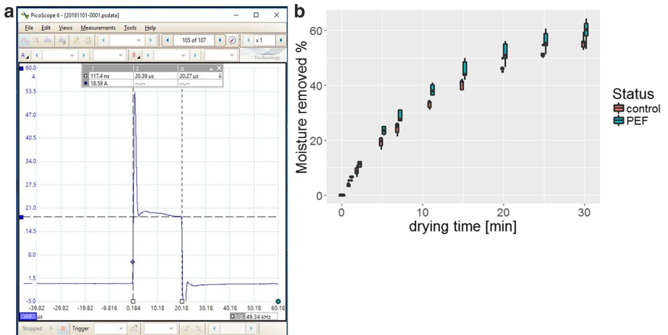
**Fig. 3** **a** The experimentally measured oscillogram of a 20- $\mu\text{s}$  pulse with 107 V amplitude applied on a known resistor of 5  $\Omega$ . **b** Moisture removed from the chicken breast muscle. 5 repetitions of control vs 5 repetitions of PEF-treated samples
