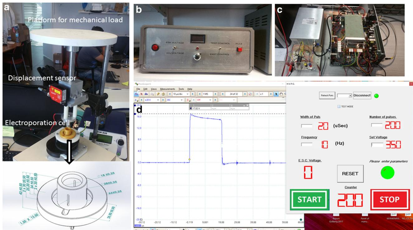
**Fig. 2** The developed pulsed electric field system for meat biomass electroporation. **a** Mechanical electroporation chamber with slider electrodes. **b** Pulse generator box. **c** Digital image of the assembled pulse generator components. **d** Controlling software interface
