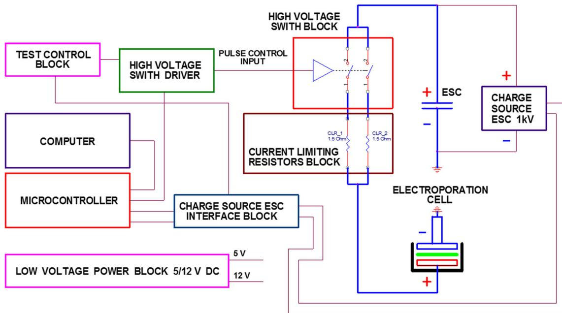
Fig. 1 Functional scheme of the high-voltage pulse electric field generator
