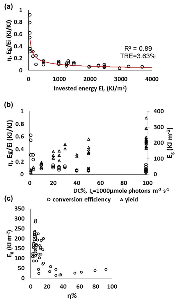
**FIGURE 5** (a) Exergy efficiency of light conversion to chemical energy vs Invested energy ( $E_i$ ).  $N = 59$ . (b) Exergy efficiency of light conversion to chemical energy and measured yield (gained energy) versus DC at a constant illumination of  $I_s$  of  $1,000 \mu\text{mole photons m}^{-2} \text{s}^{-1}$ .  $N = 55$ . (c) Yield (gained energy) versus conversion efficiency.  $N = 59$
