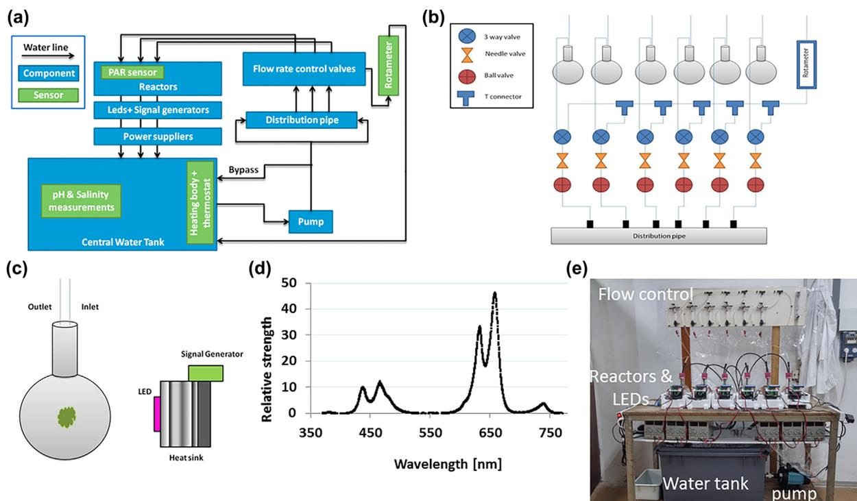
**FIGURE 1** (a) The schematic design of the laboratory scale macroalgae photobioreactor for macroalgae cultivation under the pulsed light. (b) Schematic design of a flow regulation system. (c) Schematic presentation of a single reactor. (d) Measured spectrum of used LEDs. (e) Digital image of the developed laboratory macroalgae photobioreactor
