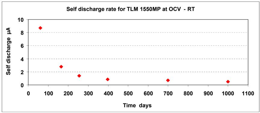
During the first 100 d the average self discharge is about 9  $\mu A$ . The value of self discharge is decreasing to about 0.5  $\mu A$  after 1000d
