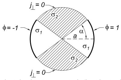
Phase 1, with electrical conductivity  $\sigma_1$ , occupies the "bowtie" region of angle  $\pm \alpha$ , while phase 2, with conductivity  $\sigma_2 \ll \sigma_1$ , occupies the remaining region.
