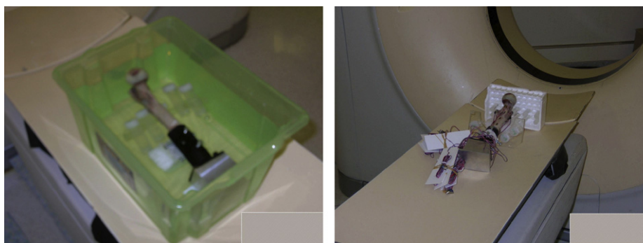
Fig. 1. Bone and K_2HPO_4 phantoms scans under two different conditions wet CT (left) and dry CT (right).
