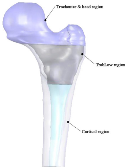
Fig. 3. The three regions of the proximal femur model. The trabecular region was divided into two sub-regions, each with a different spatial field for Young’s modulus.
