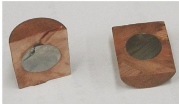
Fig. 13. Cut specimen after the experiment. The minimum and maximum diameter and height are available for comparison with the simulation.
