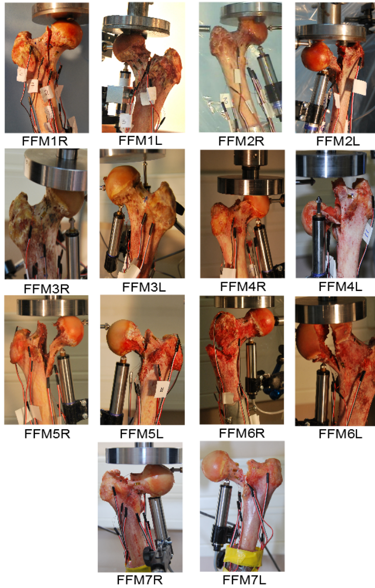
Figure 8: Fracture patterns in femurs.
