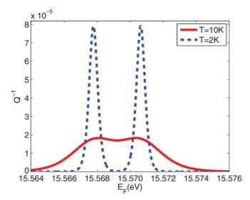
FIG. 10. (Color online) Inverse quality factor of the flexural mode  $q = 2\pi/(10^3) \text{ nm}^{-1}$  in an infinitely long beam with a = b = 10 nm at T = 2 K and 10 K as a function of the Fermi energy.
