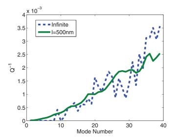
FIG. 13. (Color online) Inverse quality factor of the lowest forty flexural modes of a finite beam with  $l = 0.5 \ \mu$ m and  $a = b = 20 \ nm$  at  $T = 10 \ K$ . The results obtained for the same values of q for an infinite beam are given for comparison.
