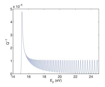
FIG. 11. (Color online) Inverse quality factor of the flexural mode  $q = 2\pi/10^3 \text{ nm}^{-1}$  in an infinitely long beam with a = b = 10 nm at T = 300 K as a function of the Fermi energy.
