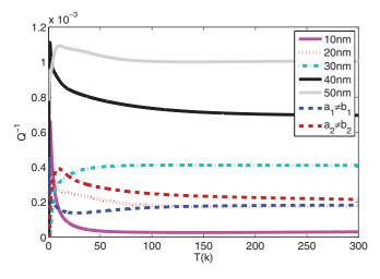
FIG. 5. (Color online) Inverse quality factor of the flexural mode  $q = 8\pi/(0.5 \times 10^3) \text{ nm}^{-1}$  in an infinitely long beam with square cross sections a = b = 10, 20, 30, 40, 50 nm, and rectangular cross sections  $a_1 = 40 \text{ nm}$ ,  $b_1 = 20 \text{ nm}$  and  $a_2 = 10 \text{ nm}$ ,  $b_2 = 20 \text{ nm}$ , as a function of temperature. Note the independence of the asymptotic value on a.
