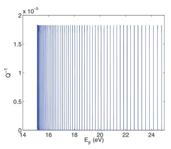
FIG. 9. (Color online) Inverse quality factor of the flexural mode  $q = 2\pi/10^3 \text{ nm}^{-1}$  in an infinitely long beam with a = b = 10 nm at T = 10 K as a function of the Fermi energy.
