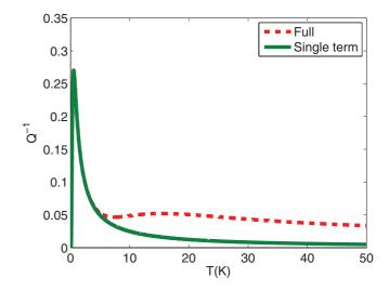
FIG. 4. (Color online) Inverse quality factor of the longitudinal mode  $q = \pi/10^3$  nm<sup>-1</sup> of an infinitely long beam with a = b = 20 nm plotted as a function of temperature, showing that up to  $T \simeq 5$  K electron-phonon damping is dominated by a single dissipation channel as explained in the text.
