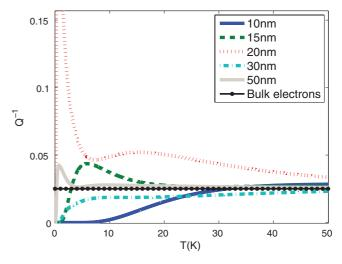
FIG. 2. (Color online) Inverse quality factor of the longitudinal mode  $q = \pi/10^3$  nm<sup>-1</sup> as a function of temperature in infinitely long beams with square cross sections, where the lateral confinement of the electrons is taken into account. The value of  $Q^{-1}$  for unconfined electrons is shown for comparison.
