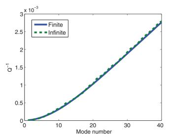
FIG. 14. (Color online) Inverse quality factors of the lowest forty flexural modes of the same beam as in Fig. 13, but at T = 300 K, compared again with the inverse quality factors of an infinite beam.
