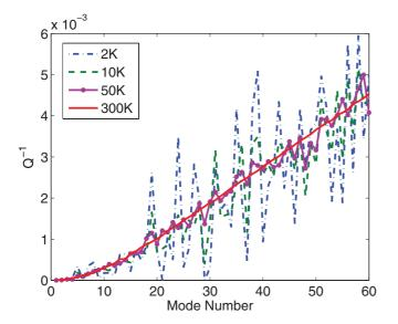
FIG. 8. (Color online) Inverse quality factor of flexural modes with  $q = \pi/(0.5 \times 10^3) \text{ nm}^{-1}$  to  $60 \times \pi/(0.5 \times 10^3) \text{ nm}^{-1}$  (which approximately correspond to the first 60 flexural modes of a  $l = 0.5 \,\mu\text{m}$  beam) in an infinitely long beam with a = b = 20 nm for different temperatures.
