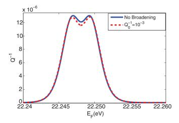
FIG. 12. (Color online) Variation of  $Q^{-1}$  of the flexural mode  $q = 2\pi/10^3 \text{ nm}^{-1}$  in an infinite beam with a = b = 10 nm at T = 10 K as a function of the Fermi energy. A solid (blue) line shows the results obtained if one ignores other damping mechanisms, while a dashed (red) line shows the results obtained using a broadened phonon spectral function in the form of a Lorentzian with  $Q_0^{-1} = \Gamma/\hbar\omega_q = 10^{-3}$ .
