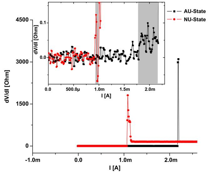
**Fig. 3.** Differential resistance of a 3 μm wide stripe in the AU-state and the NU-state at 1.5 K. The AU-state and NU-state have critical currents of  $I_{c,AU} = 2.2$  mA and  $I_{c,NU} = 1.1$  mA. Inset – enlargement of the main figure at low voltages. The grey areas show the current ranges with flux jumps.
