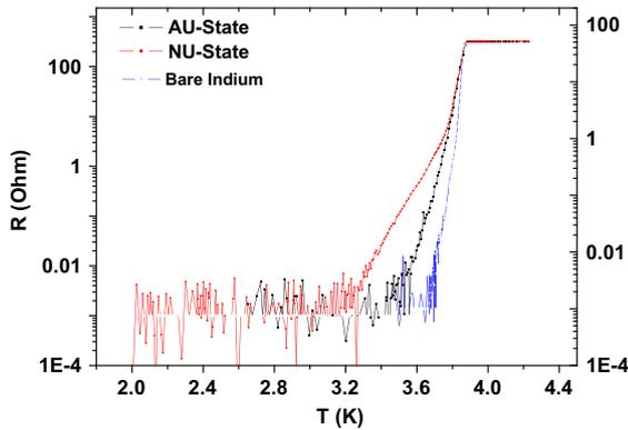
**Fig. 2.** Log scale resistance as a function of temperature for bare In and in the AU-state and the NU-state for a 3 μm stripe.
