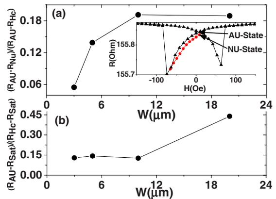
FIG. 1. (Color online) Ratios between resistances showing that when the stripe width falls below 10  $\mu\text{m}$ , the stripe is approaching the size of a magnetic domain. The inset is a measurement of the resistance as a function of magnetic field at 4.2 K for a 5  $\mu\text{m}$  stripe. It shows how the AU state and the NU state, indicated by the arrows, are reached.
