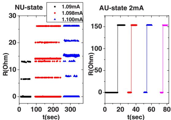
FIG. 3. (Color online) Voltage as a function of time for a 3  $\mu\text{m}$  stripe at constant currents close to  $I_c$  in the two states. The voltages are divided by the current being driven and are shown in units of ohms. (Left panel) Discrete voltage jumps in the NU state for three different currents. (Right panel) Spontaneous transitions in the AU state at a current of 2.0 mA. The data change color every time the current was switched off and back on again.
