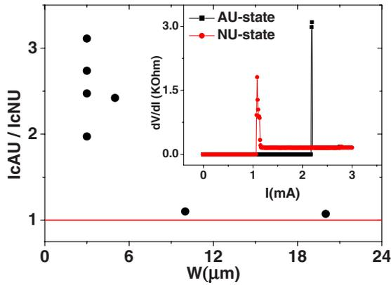
FIG. 2. (Color online) Ratio between the critical current in the AU state and the NU state as function of stripe width at 1.5 K. (inset) Differential resistance of a 3  $\mu\text{m}$  wide stripe in the AU state and the NU state at 1.5 K. The AU state and NU state have critical currents of  $I_{c,AU}=2.2$  mA and  $I_{c,NU}=1.1$  mA.
